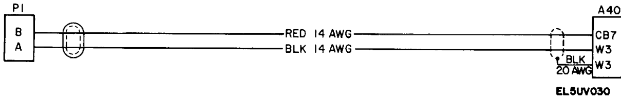
Figure 3-24. Power FM-1 cable W307A, wiring diagram.
