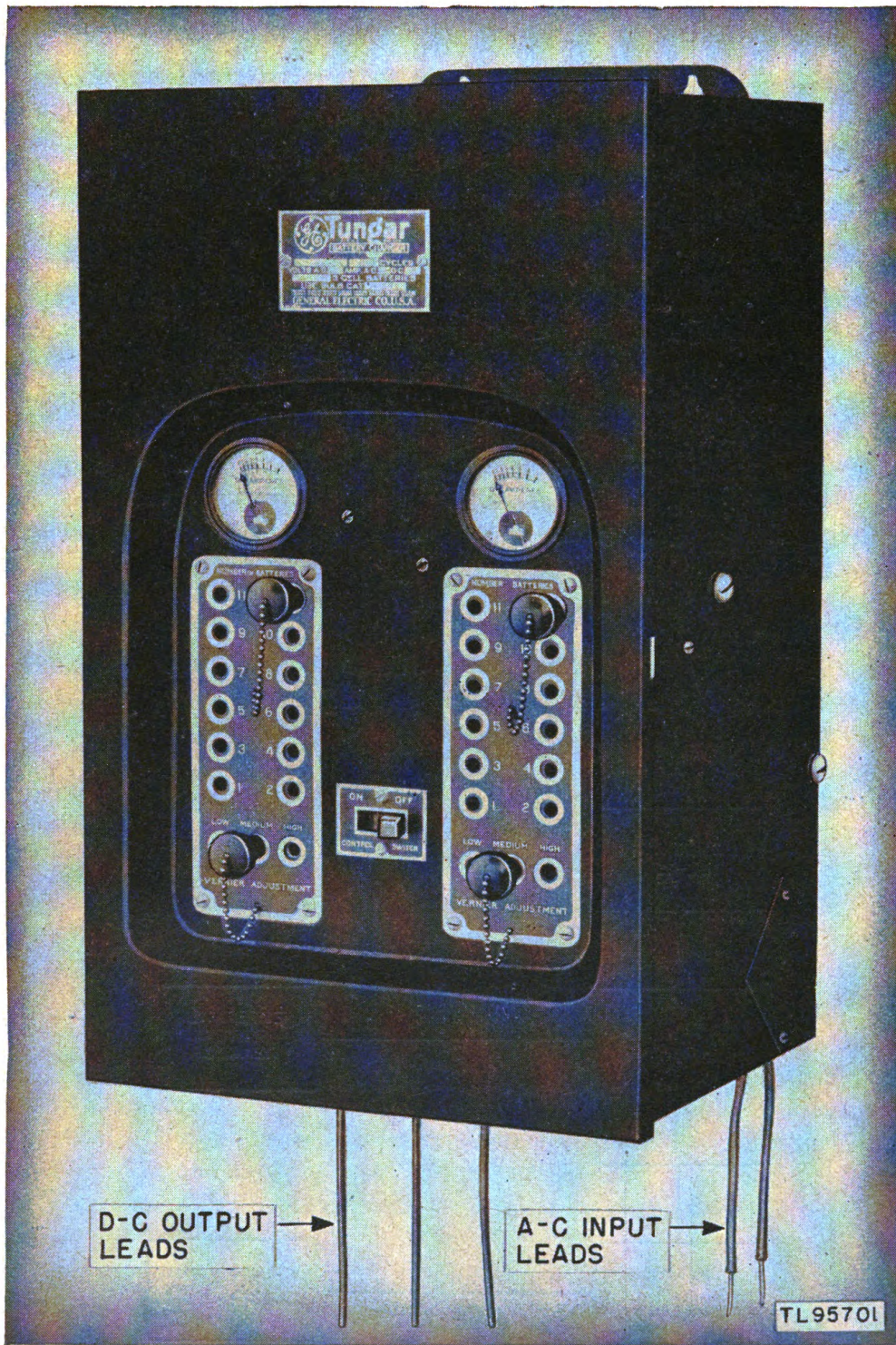
Figure 3. Rectifier 6RB6B17, showing input and output leads.
