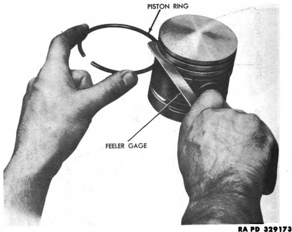
Figure 22—Checking Ring Groove Width
