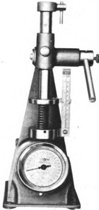
Figure 28—Checking Tension of Valve Spring With Tester (41-T-1600)
