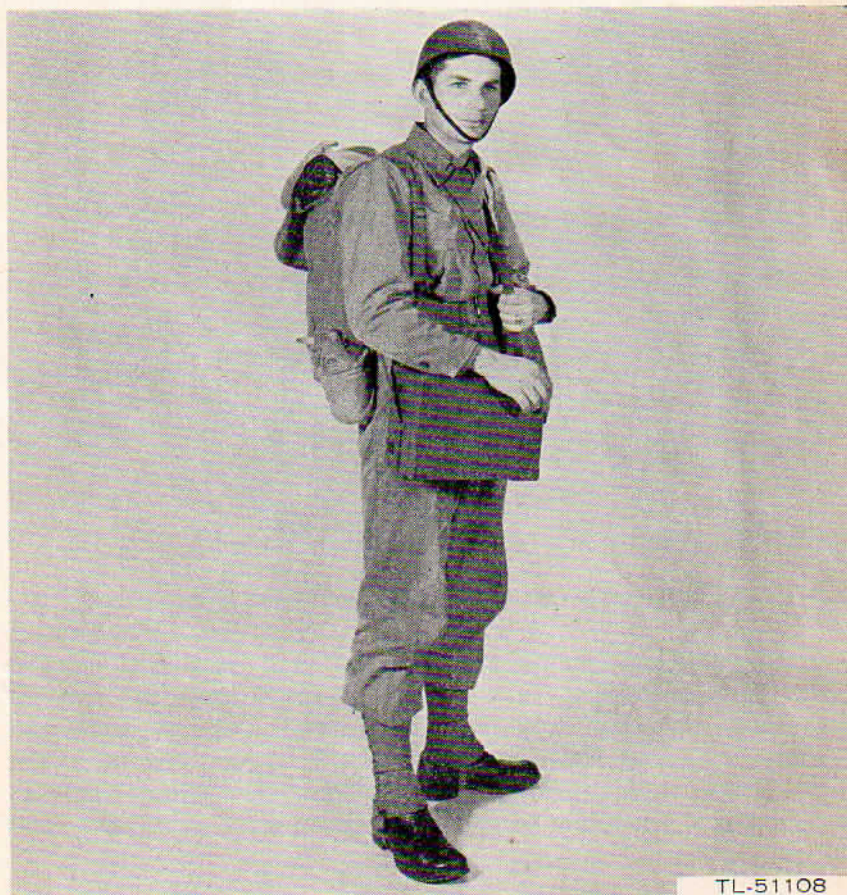
Figure 1. Switchboard SB-5/PT in carrying position.
