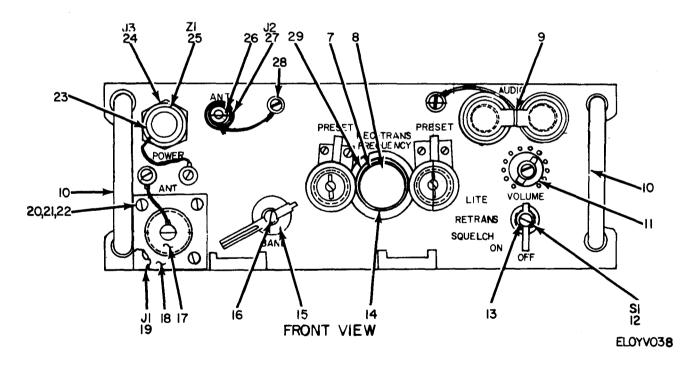
Figure 2. Panel Assembly (A30).
