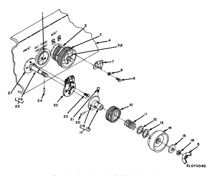
Figure 3. Panel Assembly (A30), Knob Assembly.
