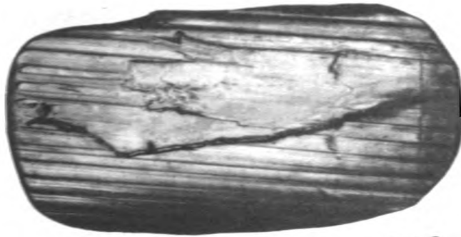
DAMAGE CAUSED BY A LOW ORDER "PREMATURITY" 1.2 IN. GUN M1895
