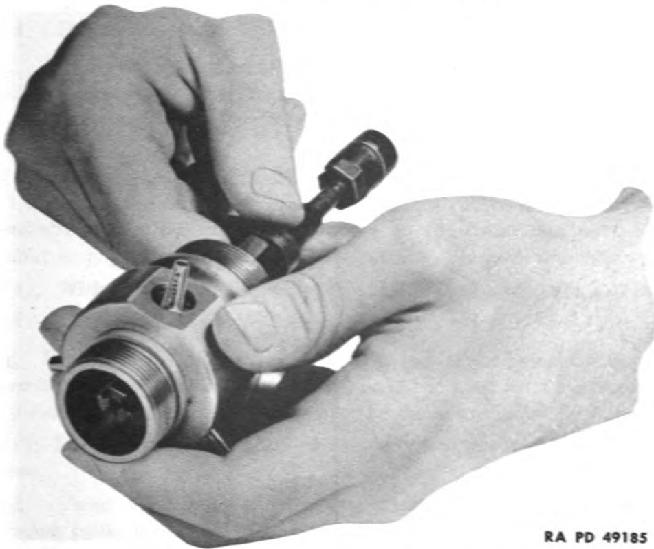
Figure 14—Assembling Head with Carriers and Points on Wedge (2-inch Star Gage)
