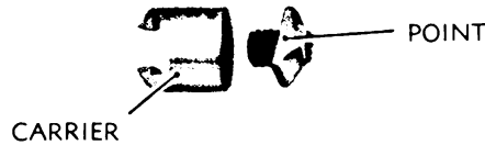
CARRIER AND SOLID MEASURING POINT FOR 20-MM GUN (0.75-INCH GAGE)
