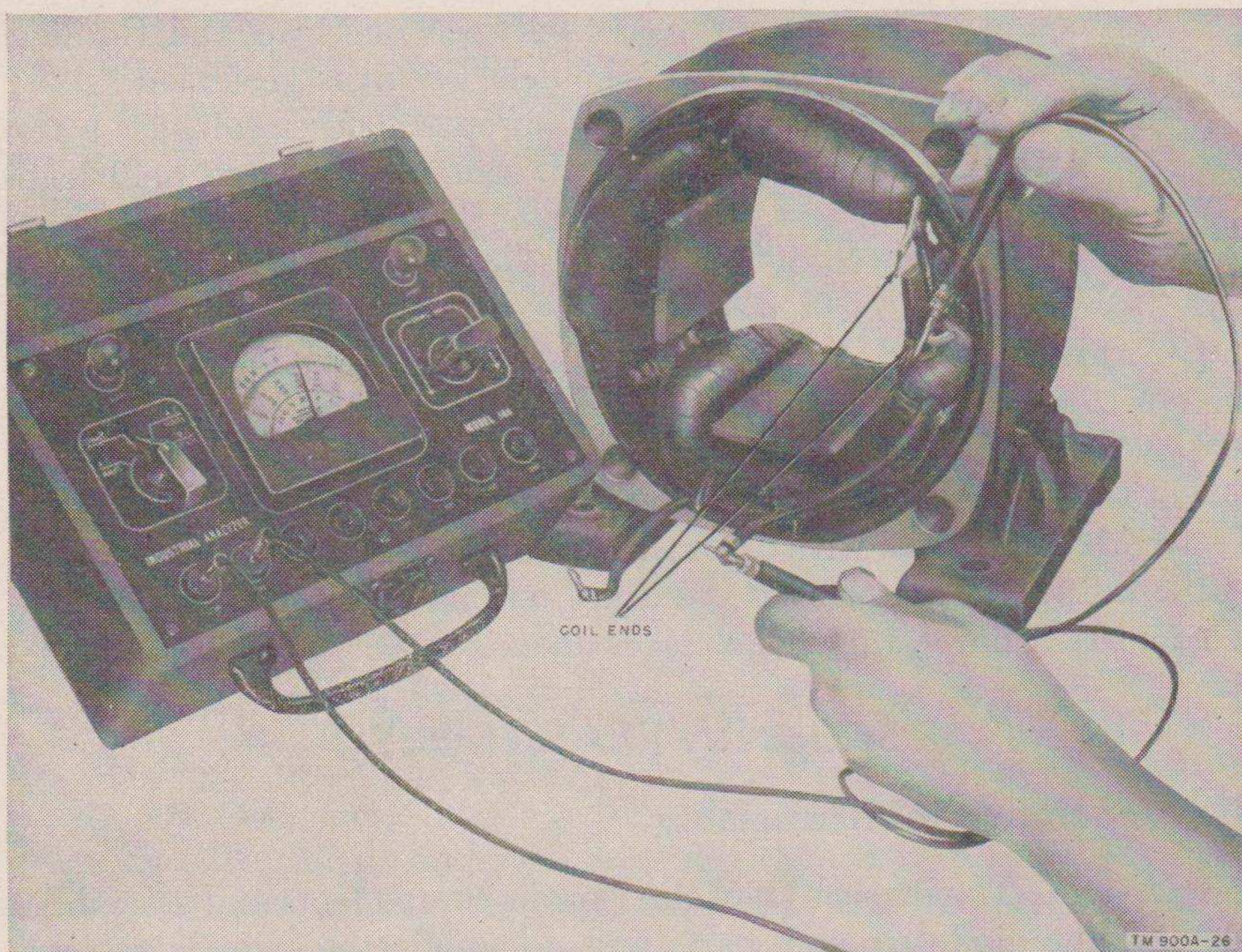
Figure 26. Testing individual field coils.
