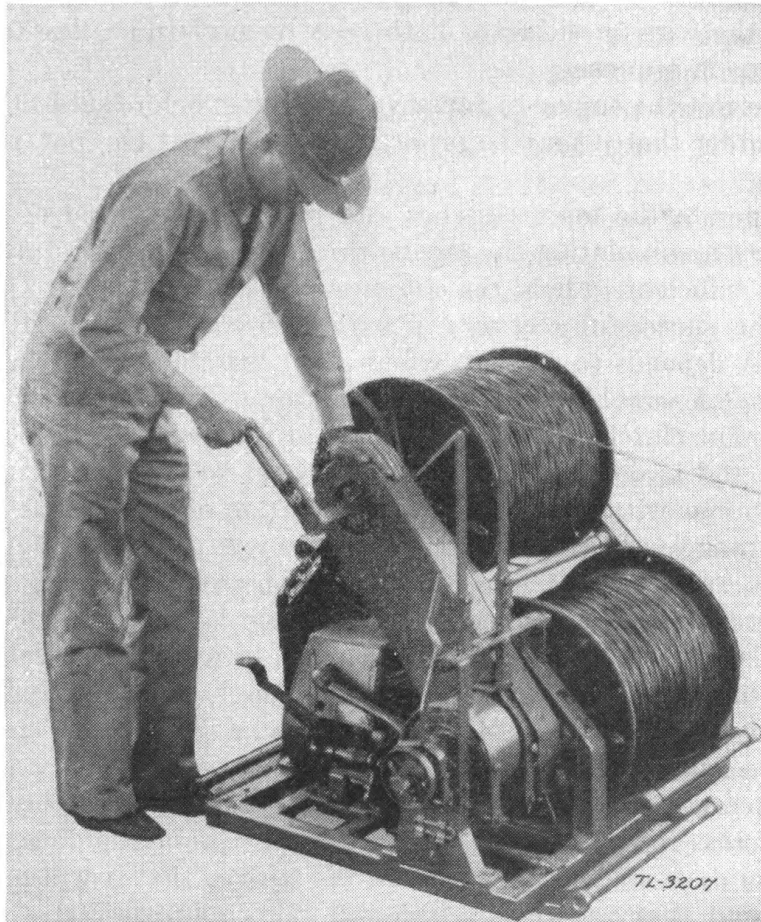
FIGURE 12.—Recovering wire on the upper reel of reel unit RL-26 by hand crank.
