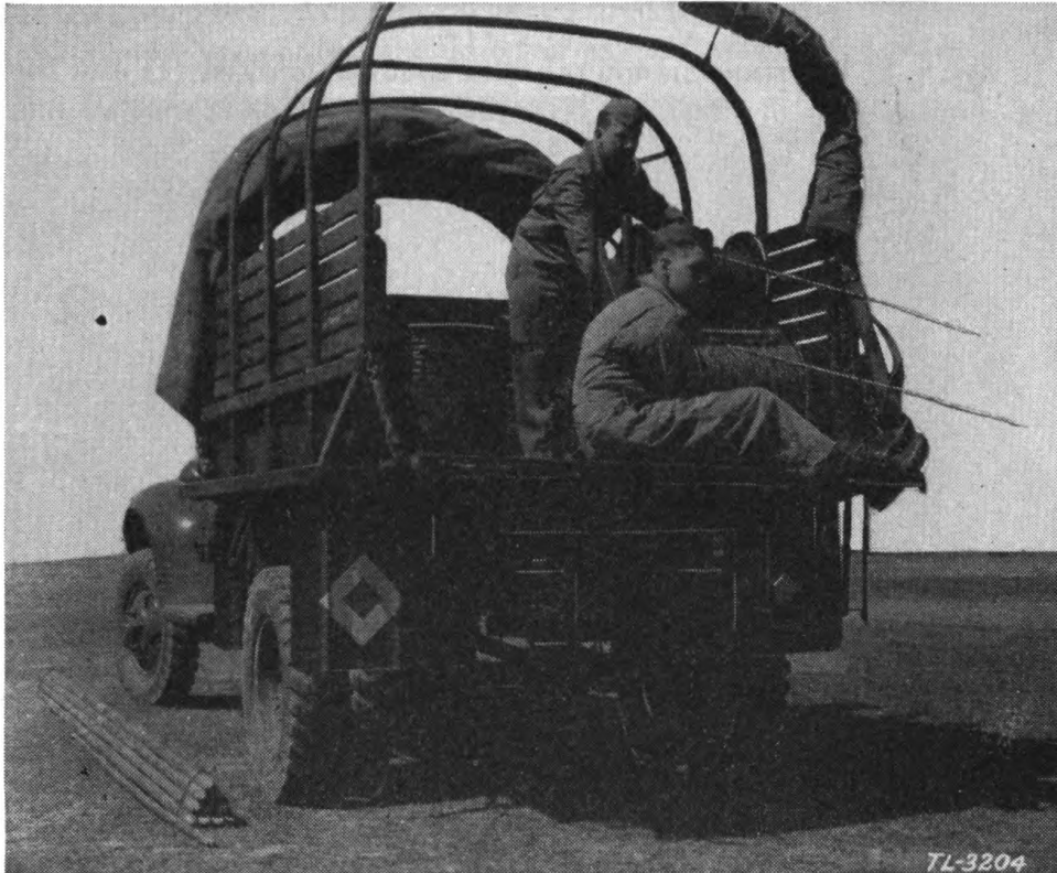
FIGURE 9.—Laying wire with truck-mounted RL-26.
