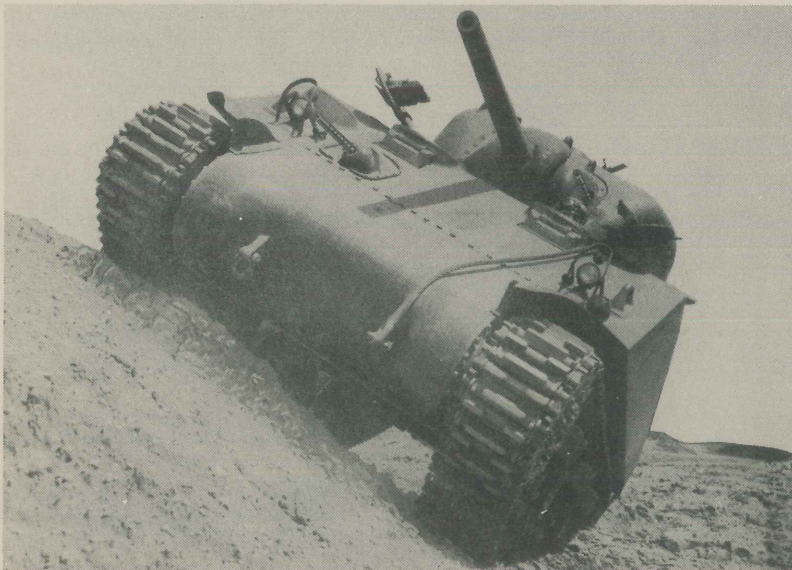
Fig. 3 - This guy defied the laws of gravity - but he broke his rear idler housing doing it.
