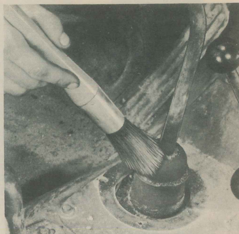
2. Take off shift lever boot and brush away all loose dirt.
