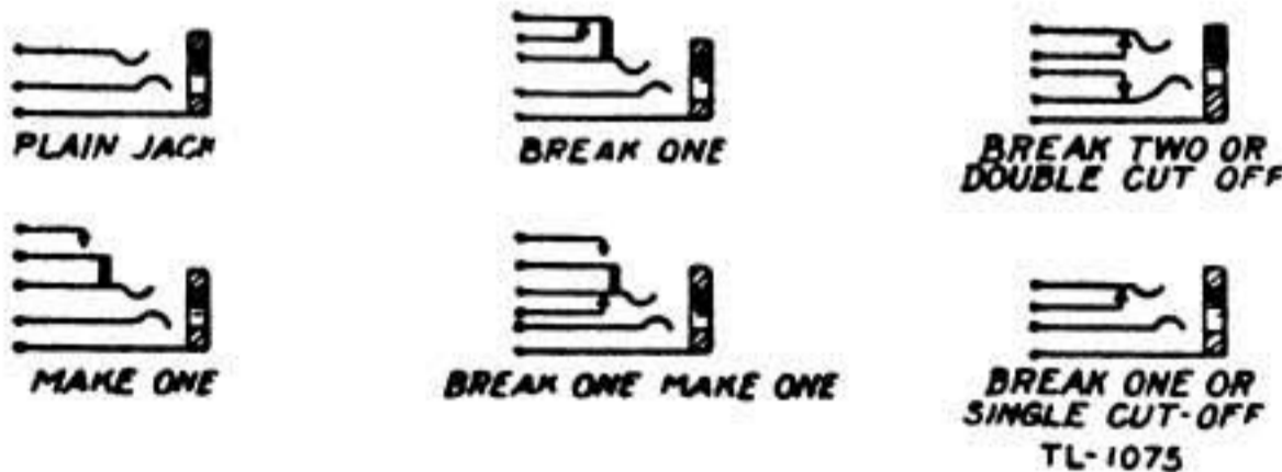
FIGURE 28.—Schematic diagrams of jacks.
