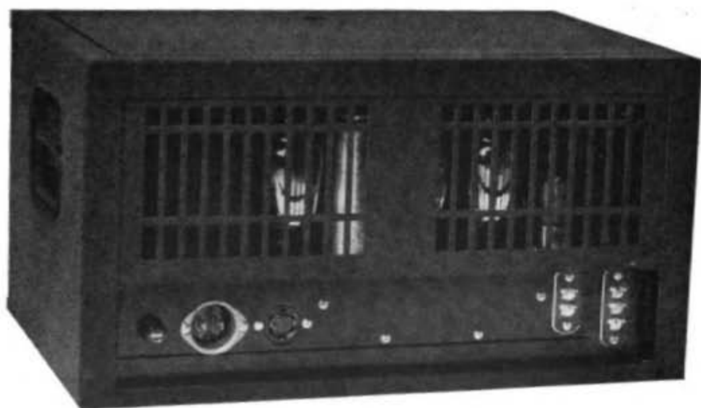
Figure 16—Recorder BC-1016, Rear View in Cabinet.
