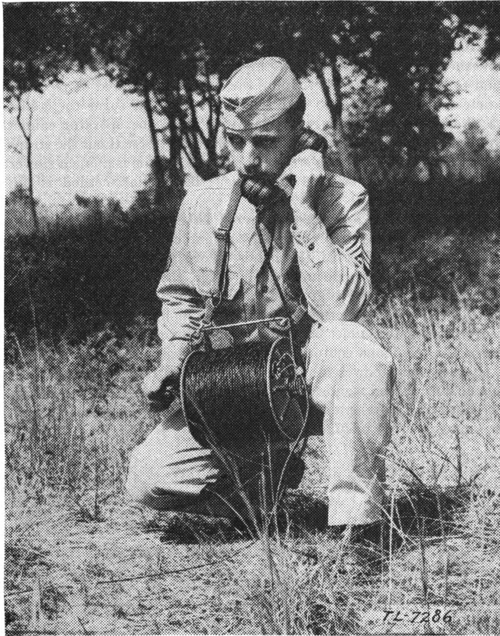
Figure 5. Using sound-powered Handset TS-10-(*) with Reel Equipment CE-11.
