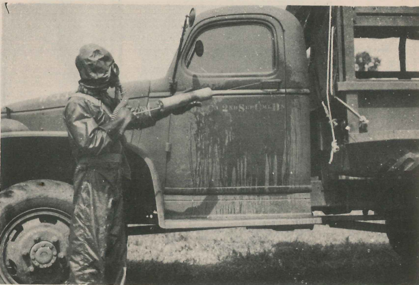
Fig. 2 - A driver all dolled-up in a Baby-Bunting (gas-proof) suit, decontaminating his poisoned truck. Chemical Warfare Service will supply the suits as needed.
