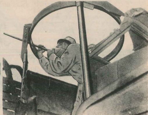
Fig. 4 - Sweeping the sky clear of enemy planes. To enable the ass't driver to fire at aerial targets, the seat cushion is taken out, the seat is thrown up, and he has a clear area of floor to dance around on. The gun ring allows a machine gun to fire in all directions.
