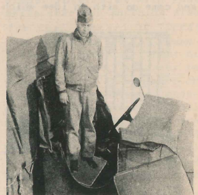
Fig. 5 - The metal platform that appears when the back of the seat folds forward. The collapsible top folds over the windshield to blackout reflections.
