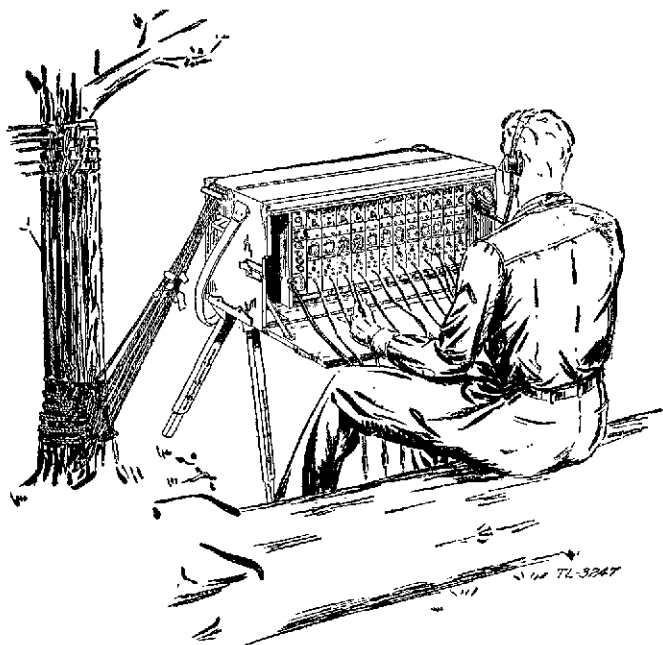
FIGURE 117.—Switchboard BD-72 set up for operation.
