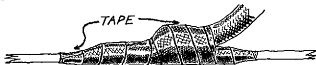
FIGURE 54.—Taping an insulated conductor spliced to bare wire.
