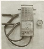
Figure 1. A battery load tester removes energy from a storage battery in much the same way starting an engine would. The experiment uses the load tester to draw the batteries down to a less than fully charged condition. DC current flow is measured using a simple hand-held low-current inductive ammeter.
