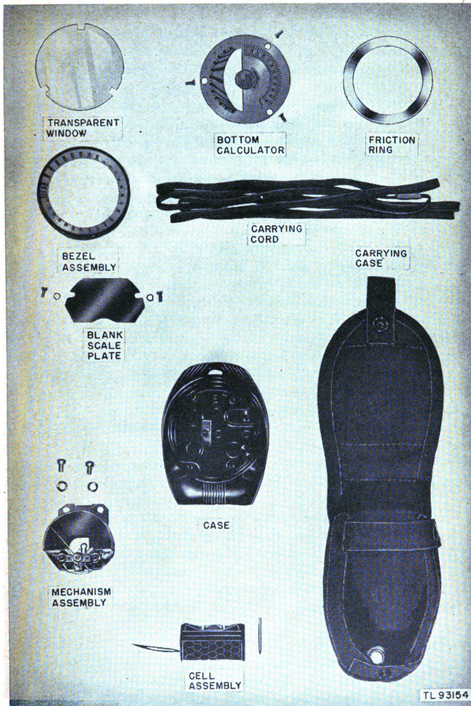
Figure 32. (Added.) Exposure Meter PH-260, disassembled.
