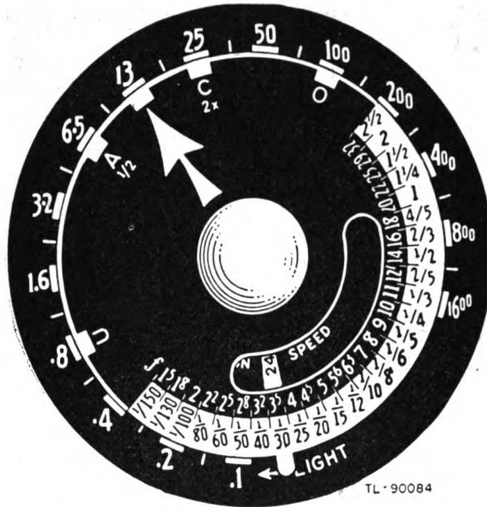
Figure 13.—Exposure Meter PH-77-C Weston M715, calculator dial with EMULSION SPEED set at 24; normal arrow at 13; A1/2 at 6.5; and C2x at 25.
