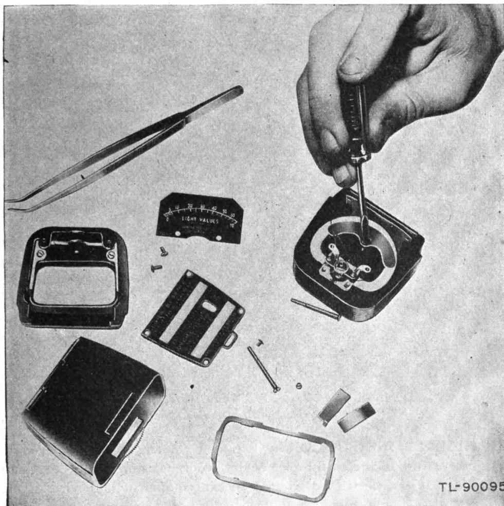
Figure 24.—Removing brace plate of Exposure Meter PH-77-C General Electric DW48.
