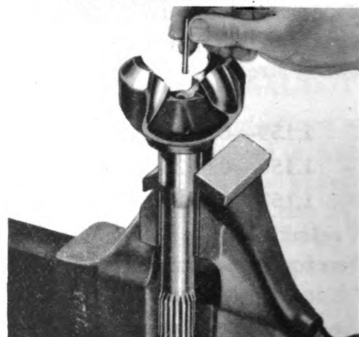
6—INSTALLING DRIVE THRUST BALL PIN
