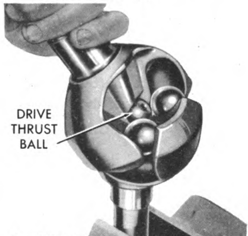
3—REMOVING OR INSTALLING UNIVERSAL DRIVE BALLS
