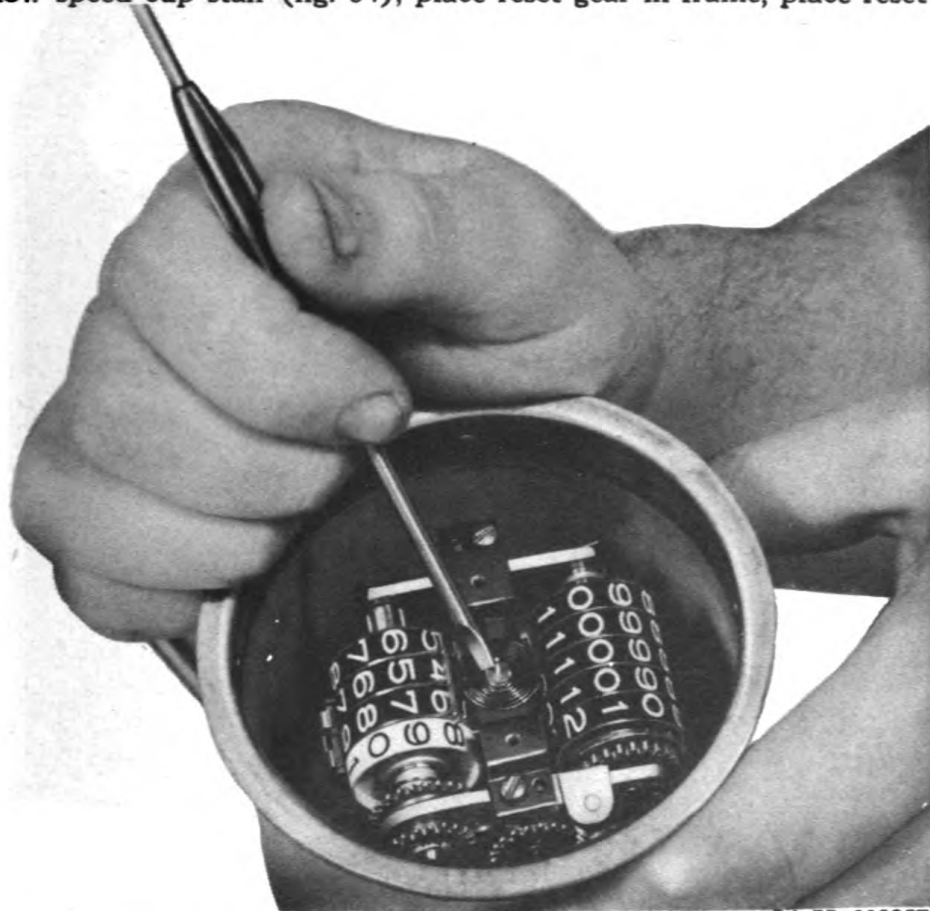
Figure 72—Adjusting Hair Spring Tension by Turning Collet on Staff, Using Adjuster (T-51742)
