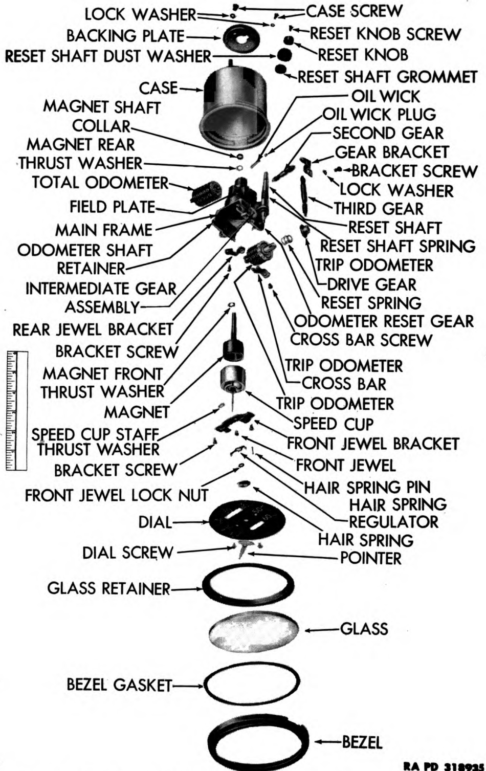
Figure 50—Stewart-Warner Speedometer with Cup-type Magnet Disassembled
