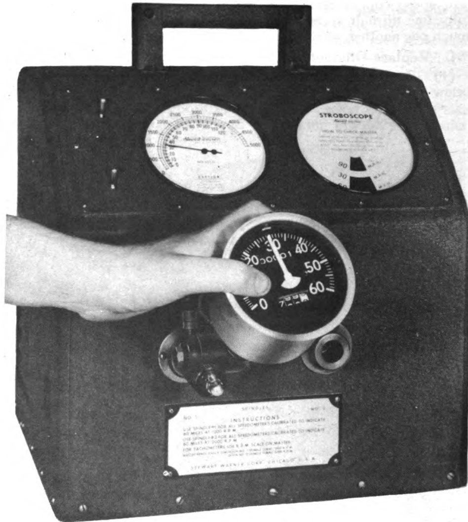
Figure 73—Holding Speedometer on Calibrating Machine (T-170645) and Testing at 30 mph
