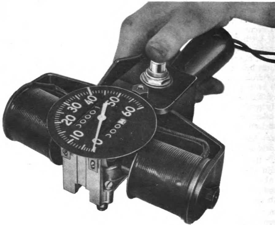
Figure 23—Charging AC Speedometer or Tachometer Magnet, Using Magnetizer (846294)
