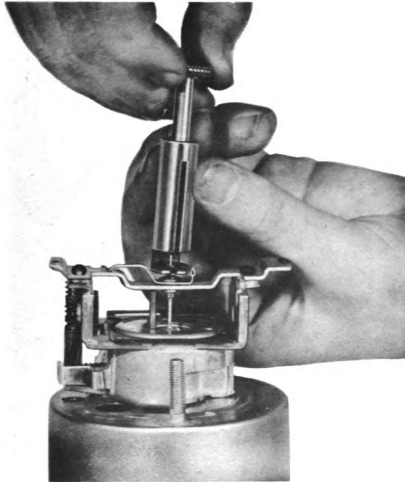
Figure 46—Removing Hair Spring, Using Puller (T-66296)
