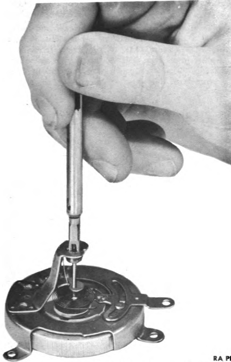
Figure 96—Adjusting Front Jewel, Using Special Tool (T-178705)
