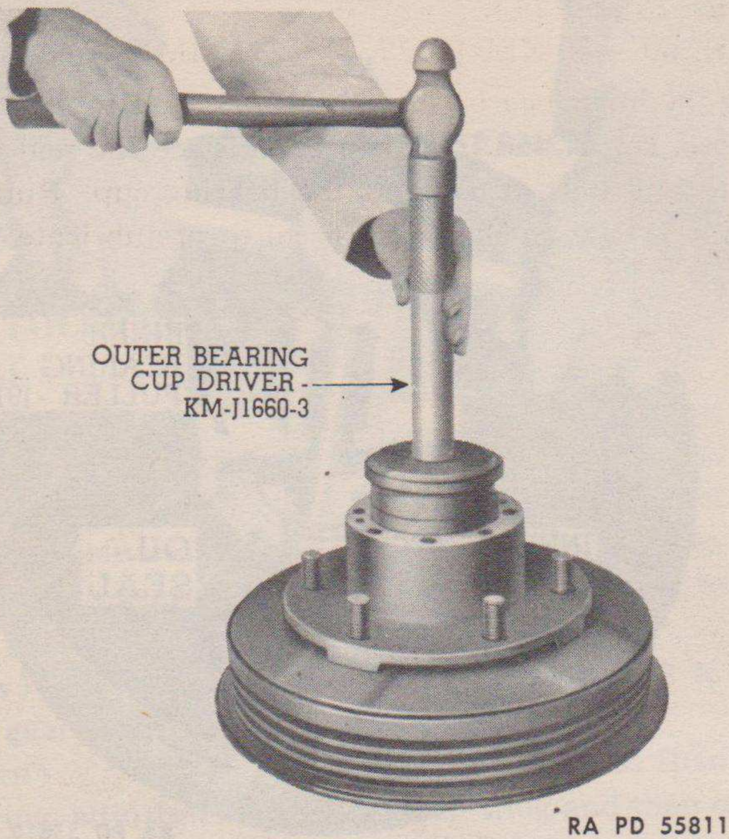
Figure 22—Replacing Outer Bearing Cup
