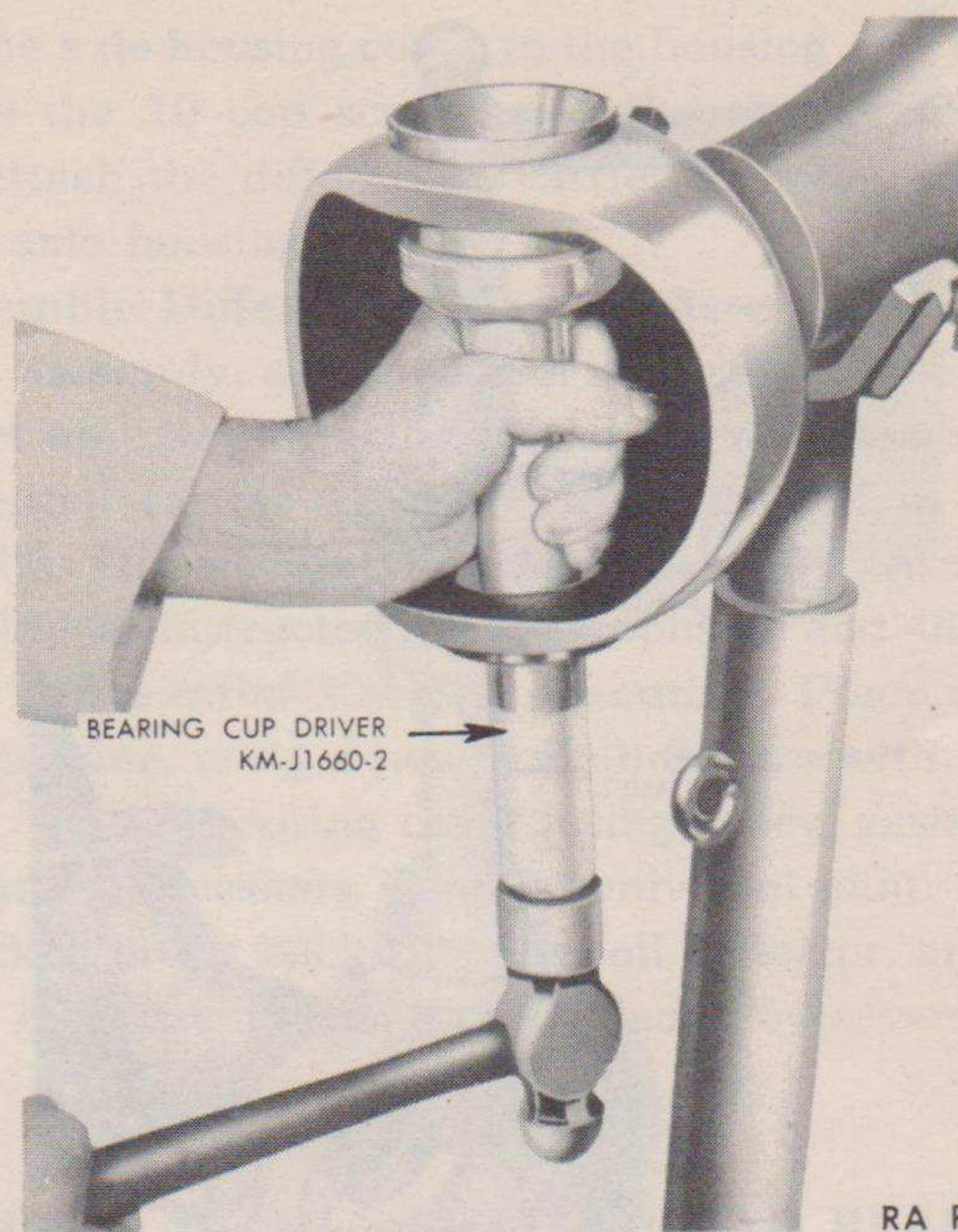
Figure 7—Removing Steering Knuckle Bearing Cup
