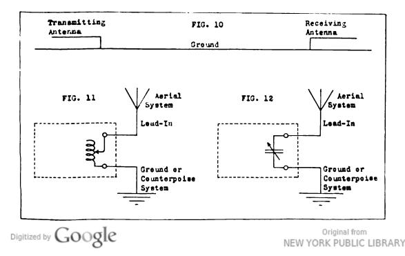
**Counterpoise Systems.**—This is by far the best method of establishing the ground side of the antenna. Instead of using a ground connection, a system of wires insulated from the ground, preferably by supporting them about 1 ft. above the ground, and run parallel and underneath the aerial wires, is employed.
