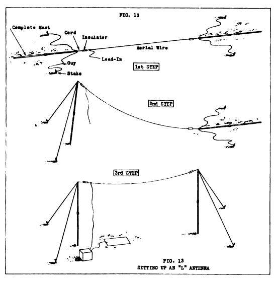
antenna poles or supports furnished with the set. In such an instance, the proper procedure is explained below, this being such as to enable one man to erect the antenna without any assistance.
