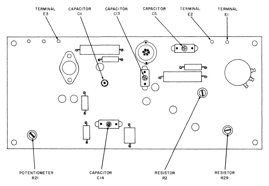
Figure 3-1. Signal Generator AN URM-127. Component Circuit Board.
