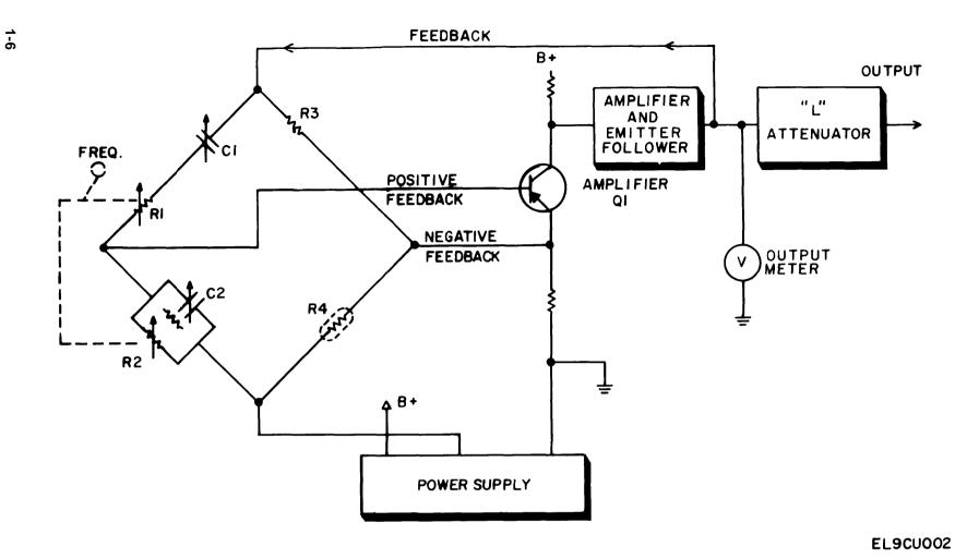
Figure 1-2. Wien Bridge Circuit.
