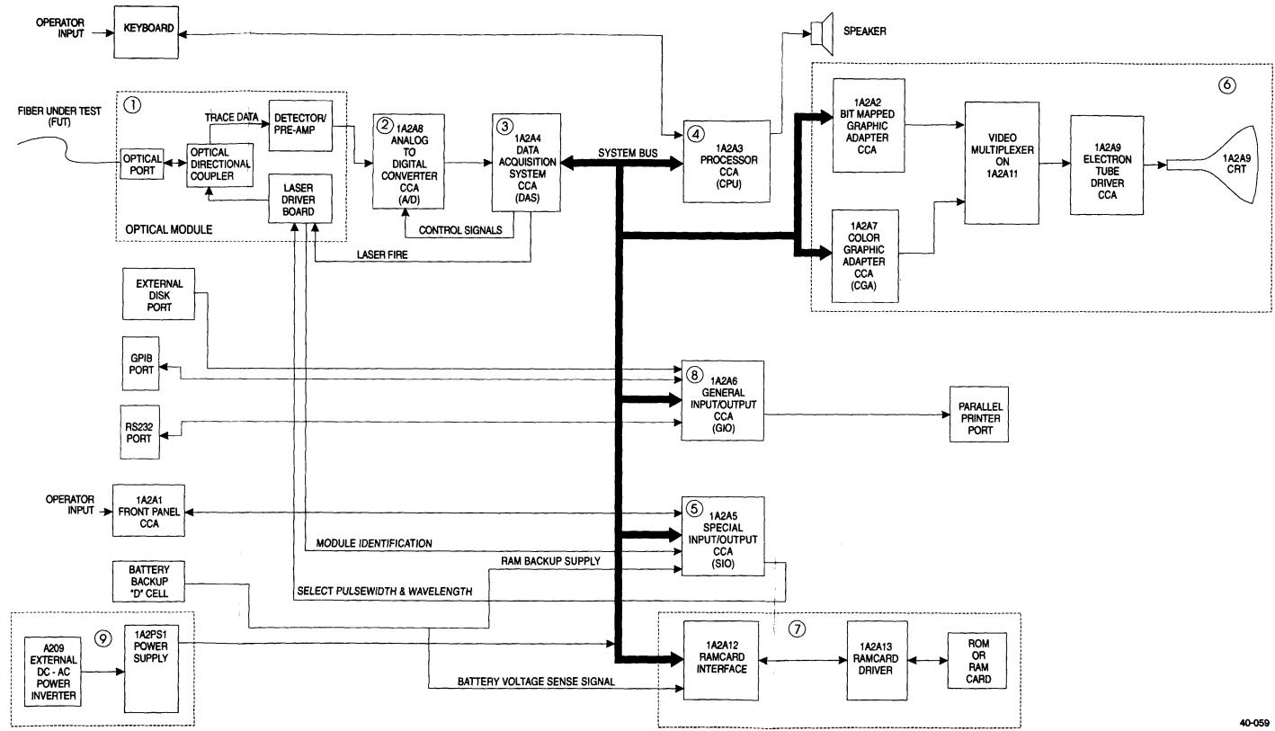
Figure FO-1. TS-4320 Functional Diagram.
