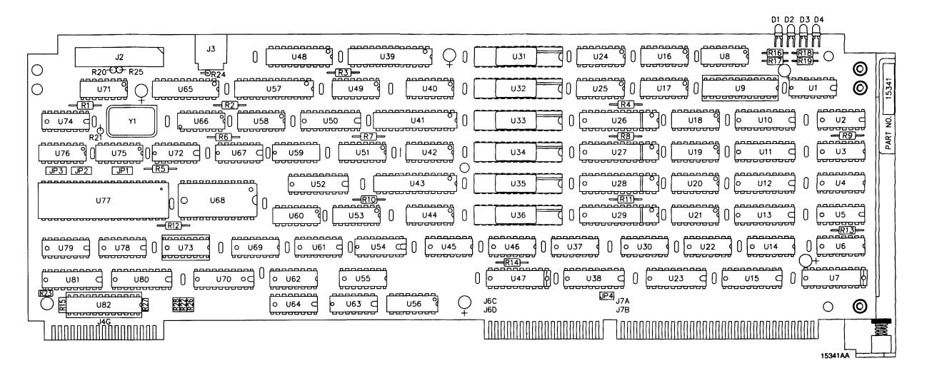
Figure FO-6. 1A2A4 DAS CCA Component Locator Diagram.
