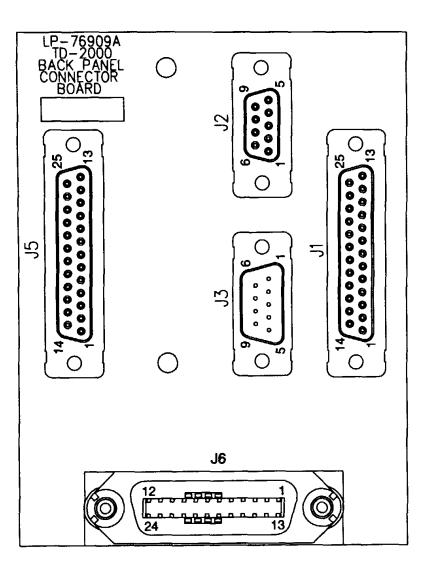
Figure FO-12. 1A2A10 Rear Panel Assembly Component Locator Diagram.
