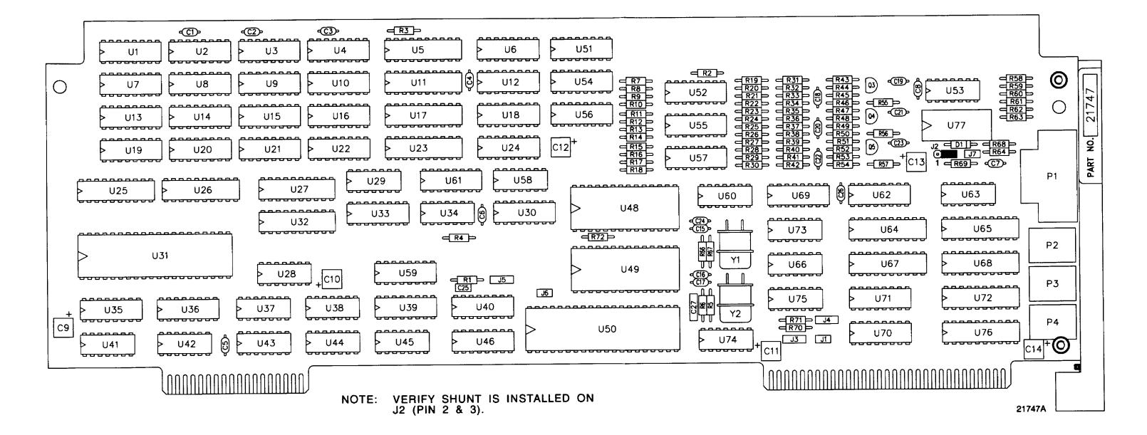
Figure FO-4. 1A2A2 Bitmapped Graphic Adapter CCA Component Locator Diagram.
