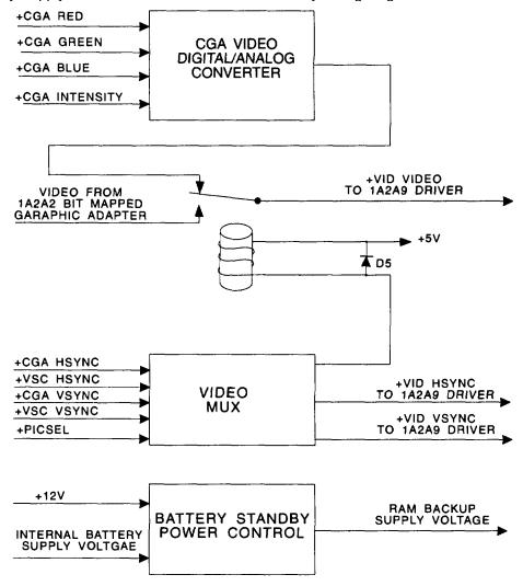
Figure 1-11. Backpanel CCA Functional Block Diagram.
