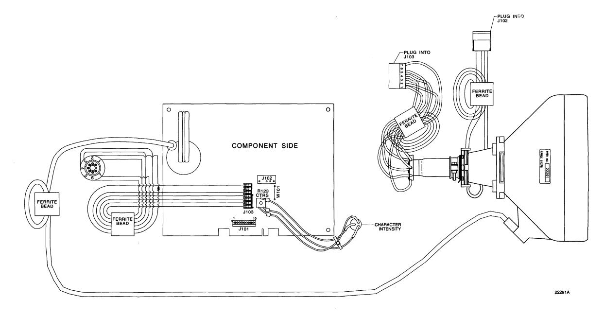
Figure FO-11. 1A2A9 Electron Tube Assembly Component Locator Diagram.
