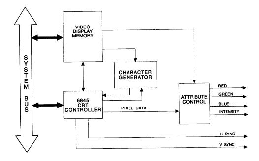
Figure 1-8. 1A2A7 Color Graphics Adapter CCA Functional Block Diagram.
