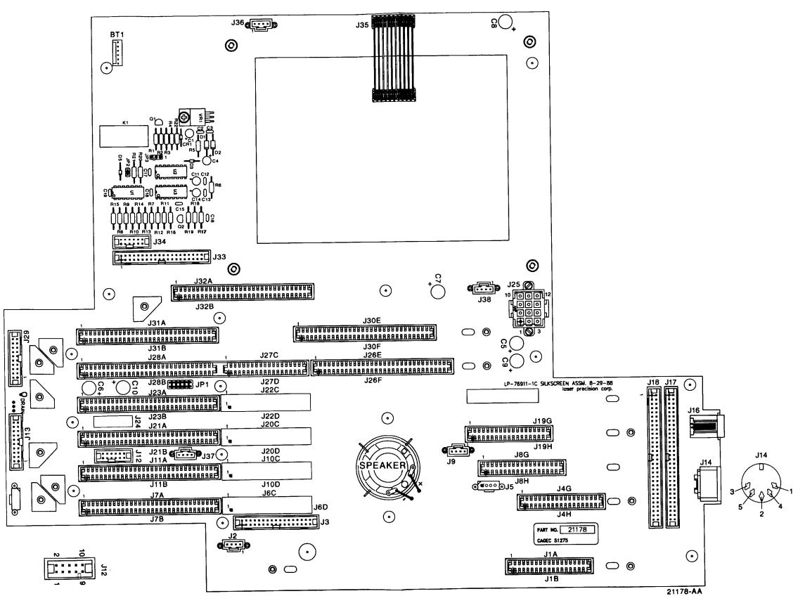
Figure FO-13. 1A2A11 CCA Backplane Component Locator & Schematic Diagram (Sheet 1 of 6).
