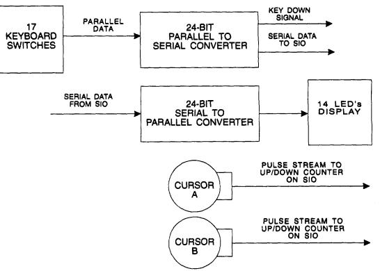
Figure 1-6. 1A2A1 Front Panel CCA Functional Block Diagram.
