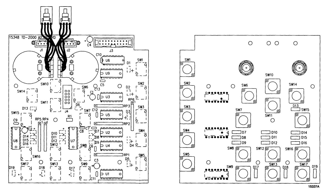
Figure FO-3. 1A2A1 Front Panel Interface CCA Component Locator Diagram.
