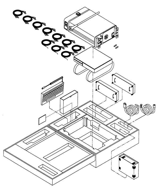
Figure 1-1. Optical Fiber Test Set TS-4320(P)/G.
