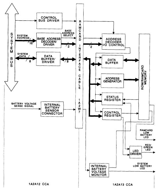
Figure 1-9. 1A2A12 RANCARD Interface CCA and 1A2A13 RAMCARD Driver CCA Functional Block Diagram.
