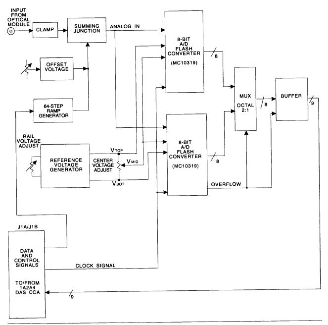
Figure 1-2. 1A2A8 A/D Converter CCA Functional Block Diagram
