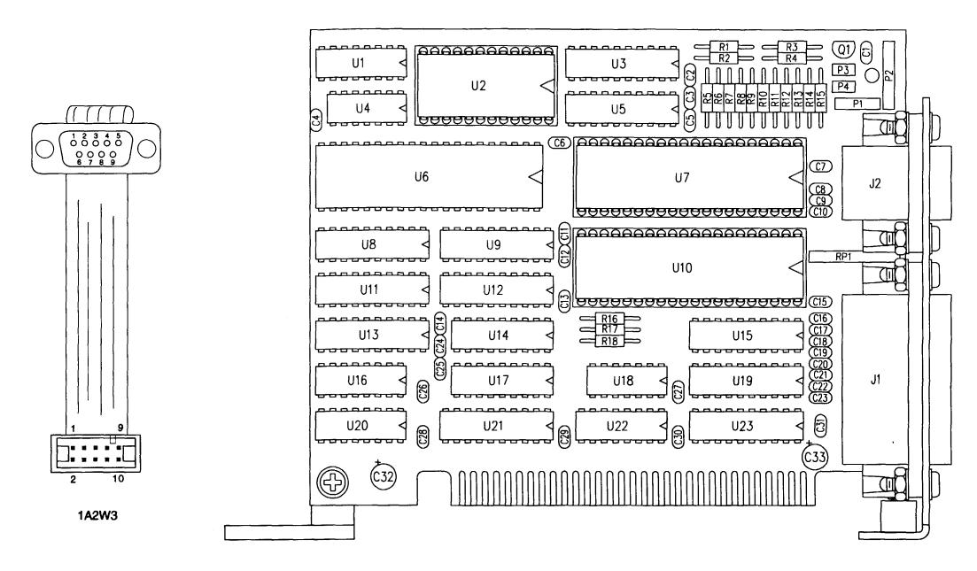
Figure FO-9. 1A2A7 Color Graphic Adapter CCA Component Locator Diagram.
