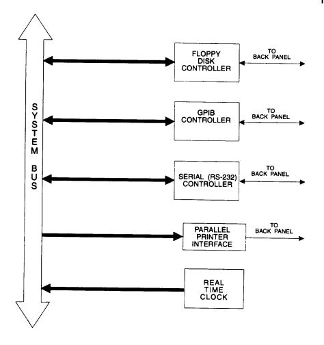
Figure 1-10. 1A2A6 GIO CCA Functional Block Diagram.
