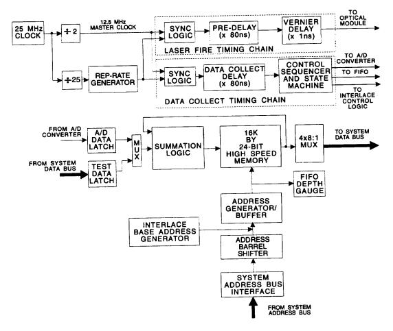
Figure 1-3. 1A2A4 DAS CCA Functional Block Diagram.
