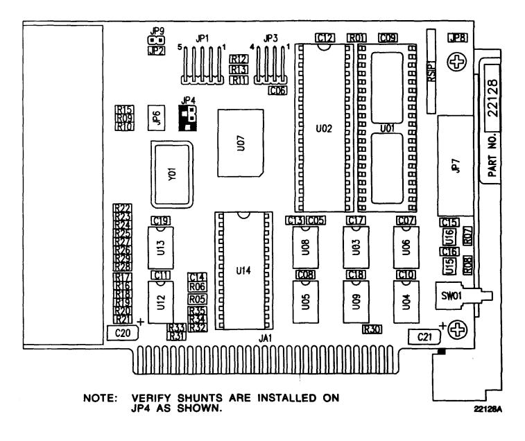
Figure FO-5. 1A2A3 Processor CCA Component Locator Diagram
