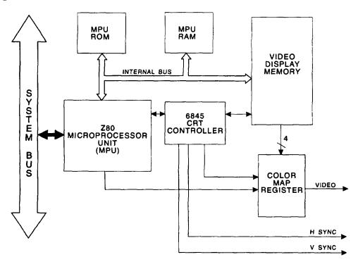
Figure 1-7. 1A2A2 Bit Mapped Graphics Adapter Functional Block Diagram.
