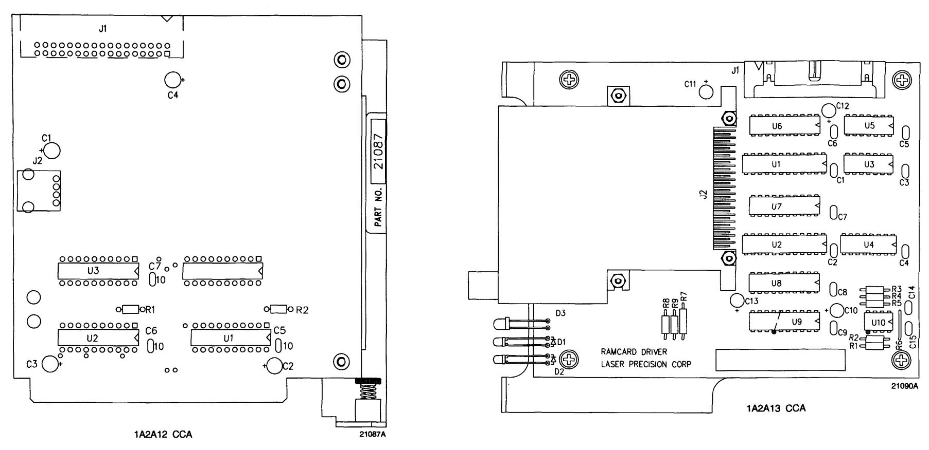
Figure FO-14. 1A2A12 RAMCARD INTERFACE and 1A2A13 RAMCARD DRIVER CCA's Component Locator Diagrams.
