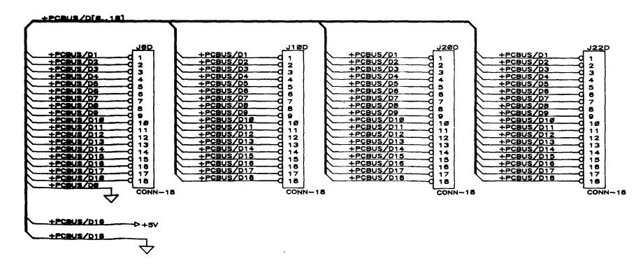
Figure FO-13. 1A2A11 CCA Backplane Component Locator & Schematic Diagram (Sheet 4 of 6).
