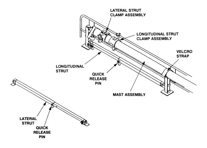
Figure 3-5. Typical Configuration of Mounting Kit Struts, Clamps, and Mast
