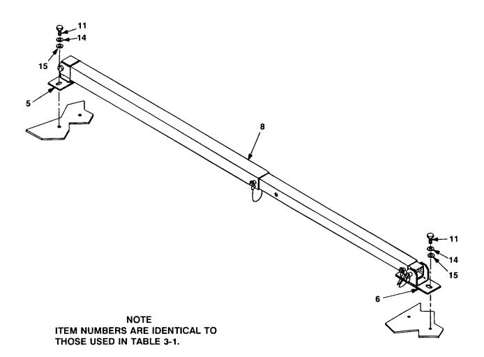
Figure 3-4. Tracked Vehicle Mounting Kit and Mast Installation (Sheet 3 of 3)
