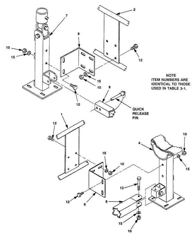
Figure 3-4. Tracked Vehicle Mounting Kit and Mast Installation (Sheet 1 of 3)
