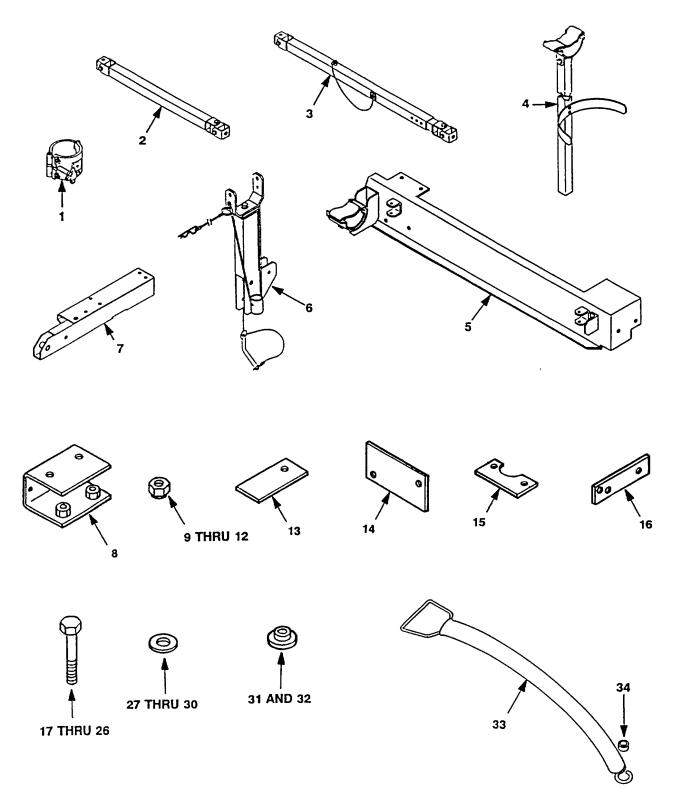
Figure 2-1. Universal HMMWV Mounting Kit Illustrated Parts
