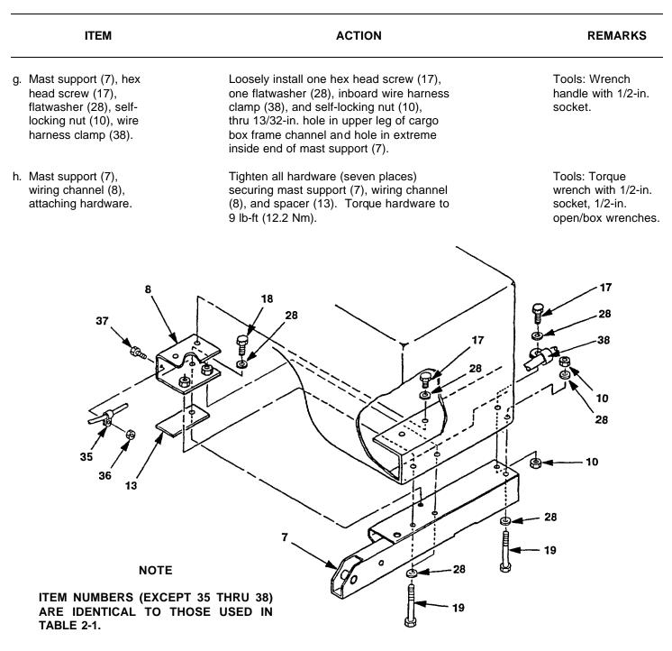
Figure 2-4. Universal HMMWV Mounting Kit and Mast Installation (Sheet 1 of 4)
