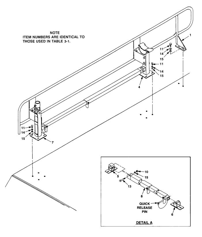
Figure 3-4. Tracked Vehicle Mounting Kit and Mast Installation (Sheet 2 of 3)
