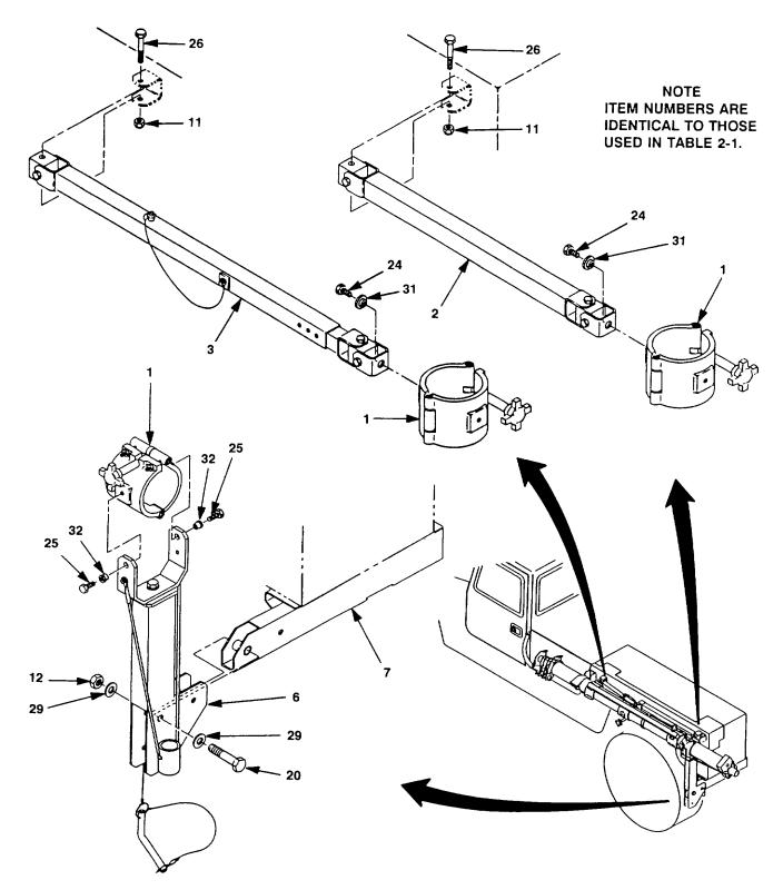
Figure 2-4. Universal; HMMWV Mounting Kit and Mast Installation (Sheet 3 of \$) 2-15
