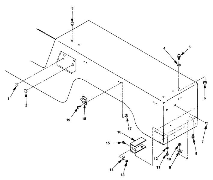
Figure 2-2. Modification of HMMWV for Mounting Universal Kit and Mast Installation **2-7**
