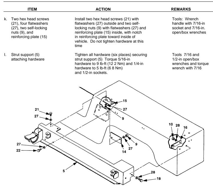
Figure 2-4. Universal HMMWV Mounting Kit and Mast Installation (Sheet 2 of 4) 2-13
