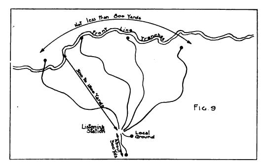
A number of grounds are installed along the first line trenches, or in no man's land as near the enemy lines as possible, Fig. 9, and each is connected to the listening station in a dugout by means of heavily insulated wire, as explained above. A local ground is also installed at the station itself and one in back of the station, about 300 yd. away. The distance between the extreme grounds should not be less than 800 yd.
