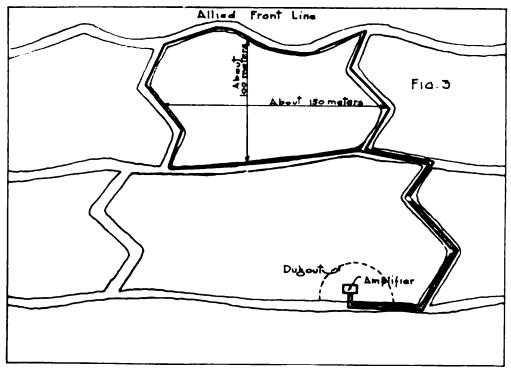
The wires connecting these grounds to the amplifier are run very close together whenever possible, either on the ground or tied by means of cords to short wooden poles, in order that the moisture on the earth's surface may not damage the insulation. No porcelain insulators are required. These wires should be run in a trench separate from that provided for the telephone and telegraph lines, so that the latter will not produce too great interference by induction.
