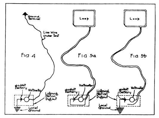
is in good condition, the voltmeter reading should be only slightly less than the direct voltage across the battery—10 per cent less perhaps. If it is more than 25 per cent below the battery voltage, the line should be examined for breaks and for poor ground connection.
