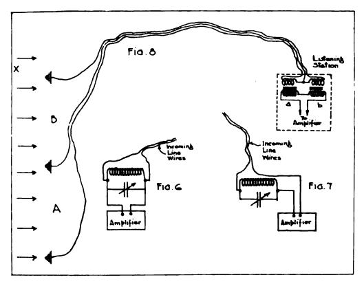
rents it is desired to receive. This circuit having higher impedance for that frequency than any other frequency, will allow most of the current to flow into the amplifier. For currents of any other frequency it will shunt most of the current. and therefore weaken the interfering noises in the amplifier.
