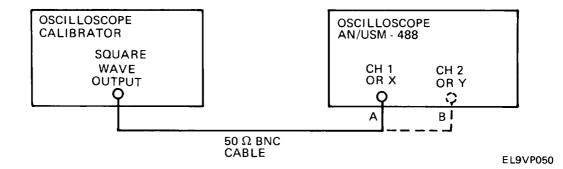
8. Select each oscilloscope channel 1 and oscilloscope calibrator setting combination listed below and verify that oscilloscope vertical deflection and accuracy is within the limits shown.
