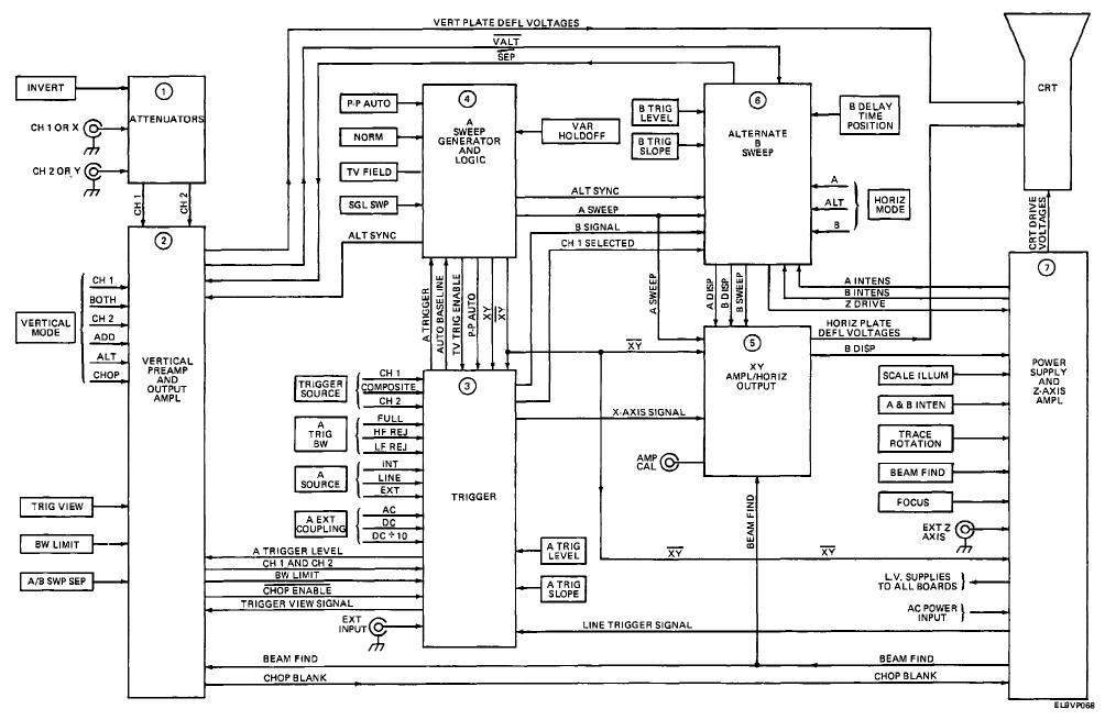
Figure FO-1. Simplified Block Diagram.
