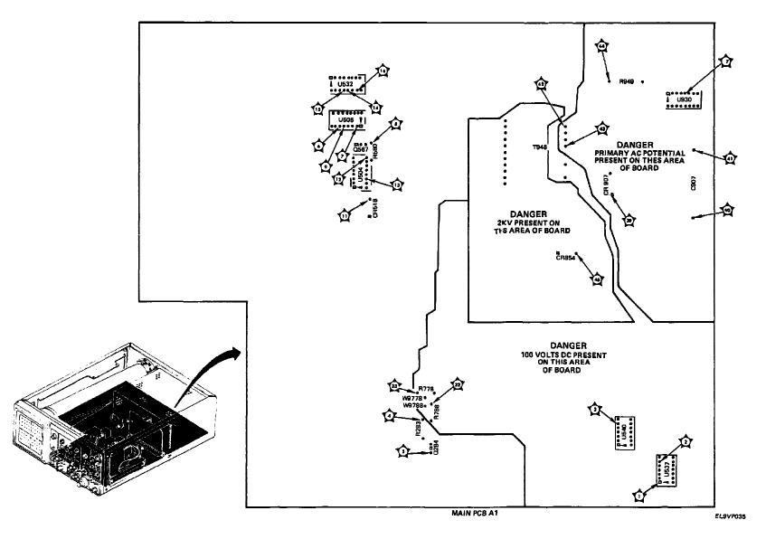
Figure FO-13. Waveform Test Point Locations (Sheet 1 of 2).
