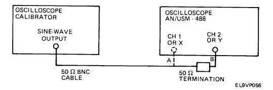
3. Set oscilloscope calibrator for 50 kHz, 6-division display.
