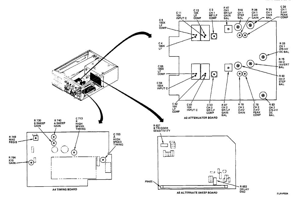
Figure FO-4. Adjustment Points (Sheet 1 of 2).
