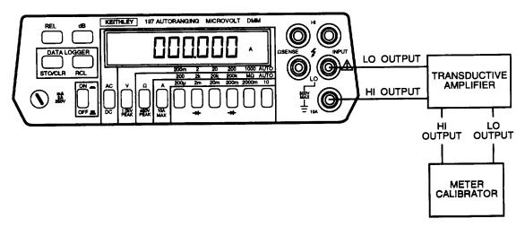
Set meter calibrator to the applied ac current (10 A) and frequencies (20 Hz through 10 kHz) as shown below. Verify
