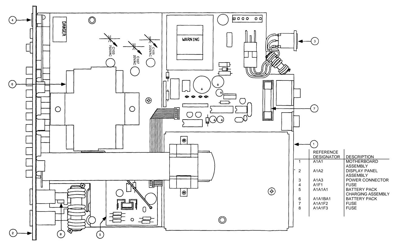
Figure FO-4. Multimeter Assembly Locator
