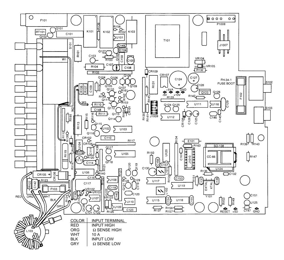
Figure FO-5. Motherboard Assembly Component Locator
