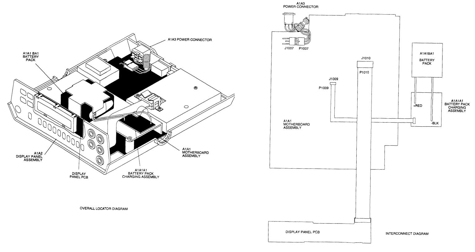
Figure FO-3. Overall Locator and Interconnect Diagrams
