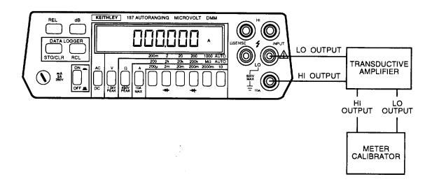
Set multimeter for each range and apply dc current as shown below. Verify that the display reads within the specified limits for each current applied. If the display does not read within all specified limits, refer to Troubleshooting (Chapter 5, Section IV).
