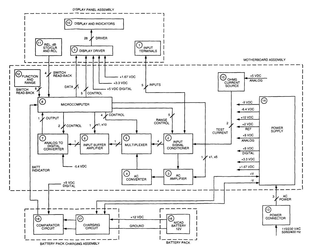
Figure FO-1. Digital Mutimeter AN/USM-486A Functional Block Diagram
