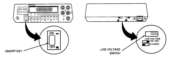
d. Set LINE VOLTAGE switch to correspond to line voltage available.
