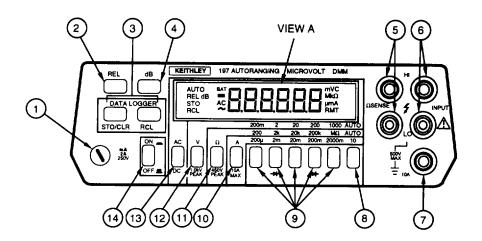
Figure 2-1. Operator's Controls, Indicators, and Connectors, Front View
