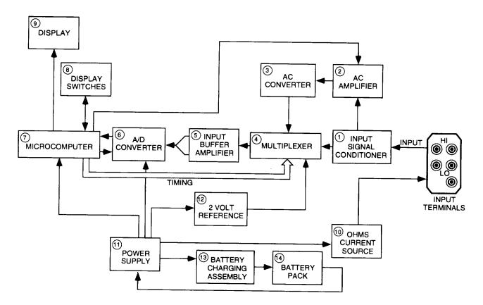
Figure 1-2. Digital Multimeter AN/USM-486A Functional Block Diagram
