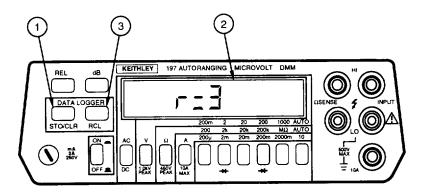
b. Press and hold in STO/CLR key (1) to scroll through the following reading rate codes on the display (2).
