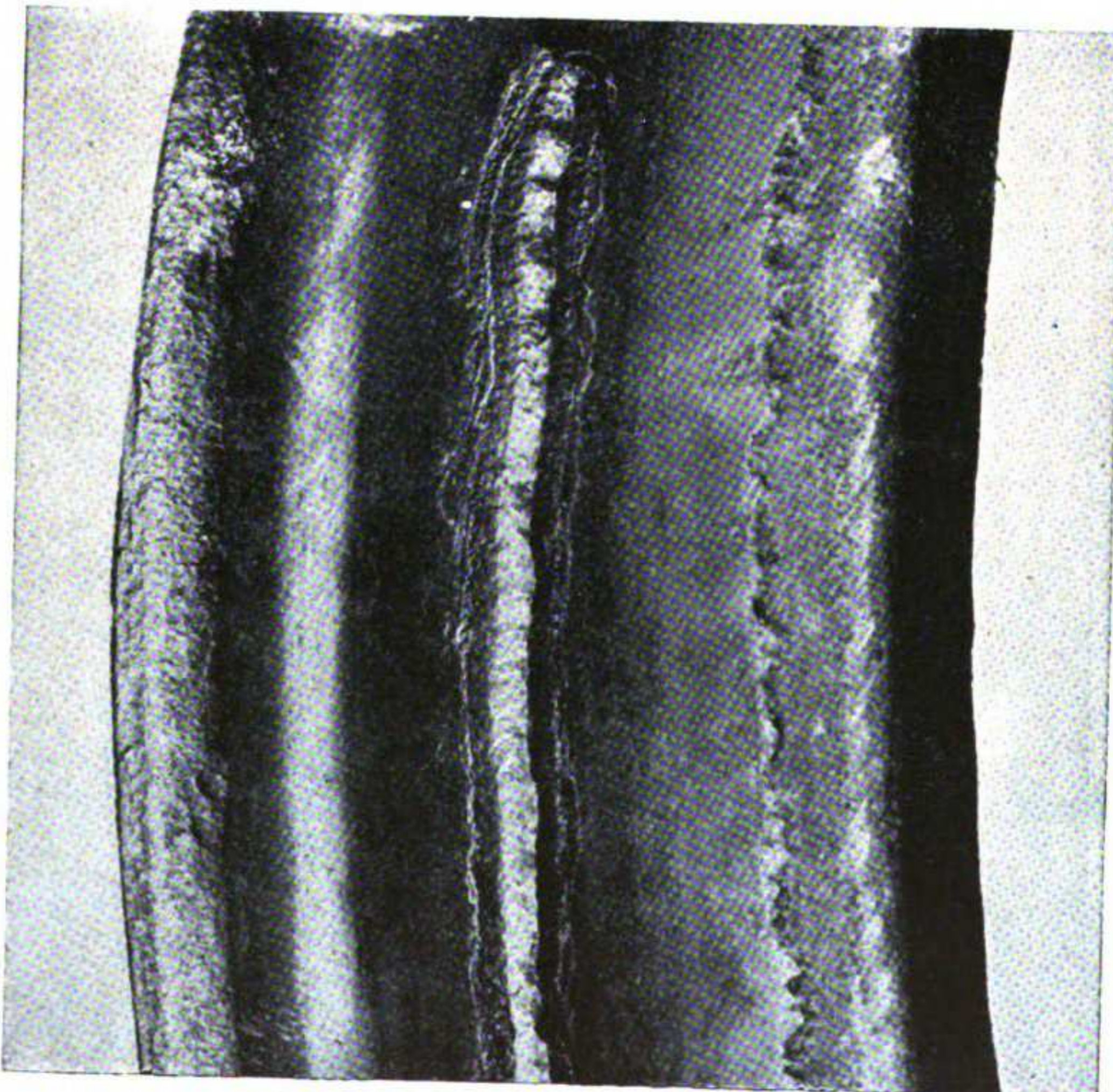
Figure 84. Seam in tread, cast-iron wheel.
