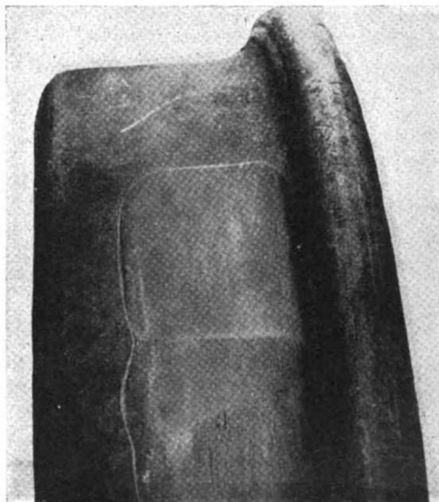
Figure 82. Double slid flat, cast-iron wheel.
