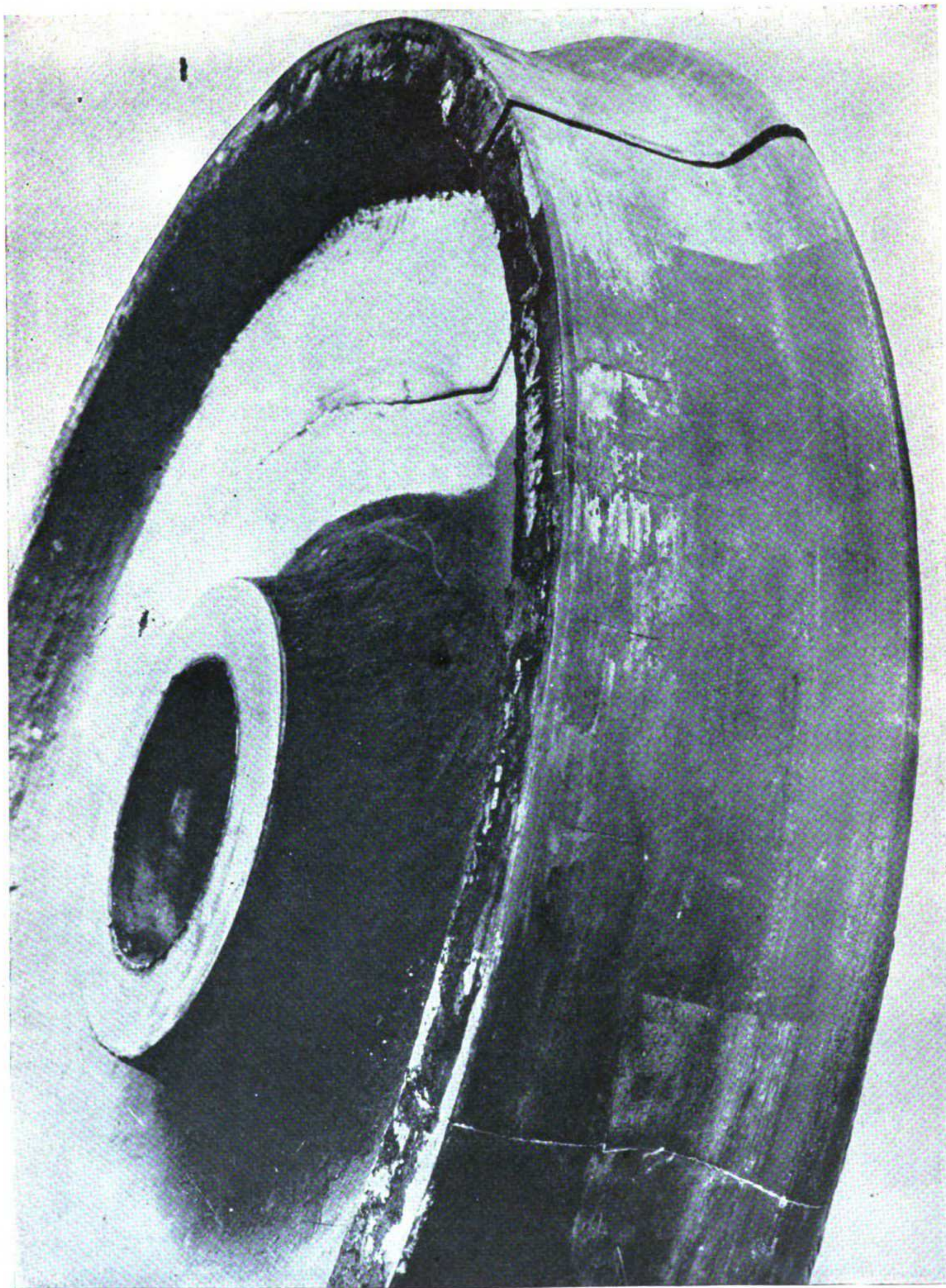
Figure 61. Wheel failure caused by thermal check.
