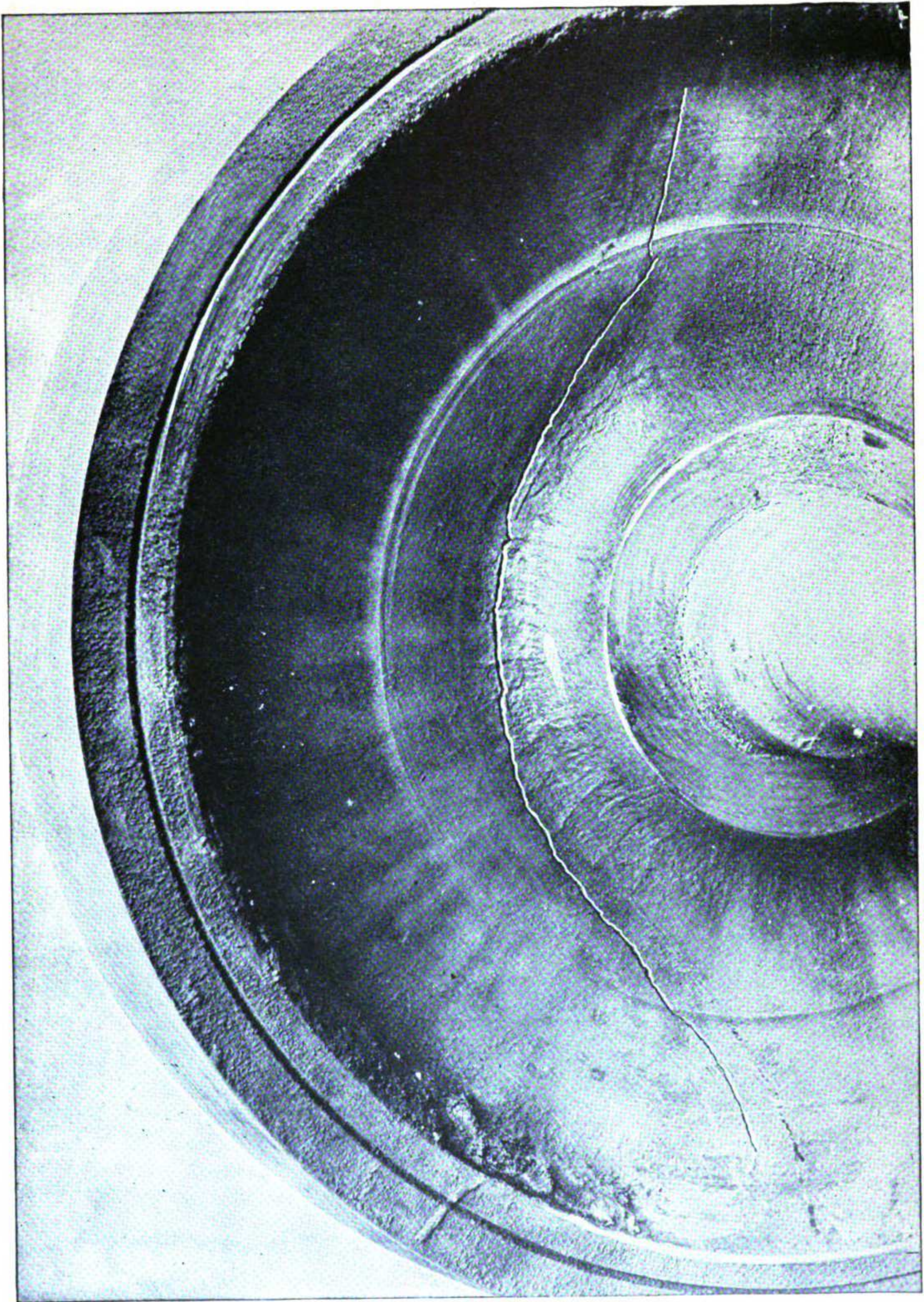
Figure 75. Circumferential crack ("Cupid's Bow" Type).
