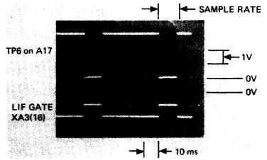
d. As the resolution is change, the width of the gate signal should vary as follows:
