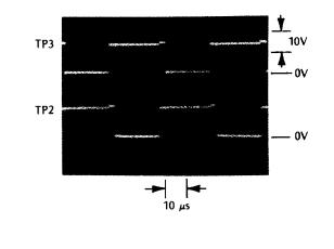
c. Connect a clip lead to A21TP4 and momentarily ground the other end to the chassis. Observe red LED turn on for approximately 1-2 seconds and waveforms at TP2, TP3 go to a constant +13 volts for same duration. If not, suspect A21U3.
