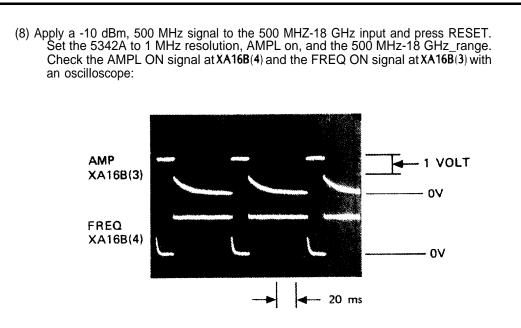
(9) If the waveforms (shown above) are not present, go to diagnostic mode 6 and check the voltages in the following table:
