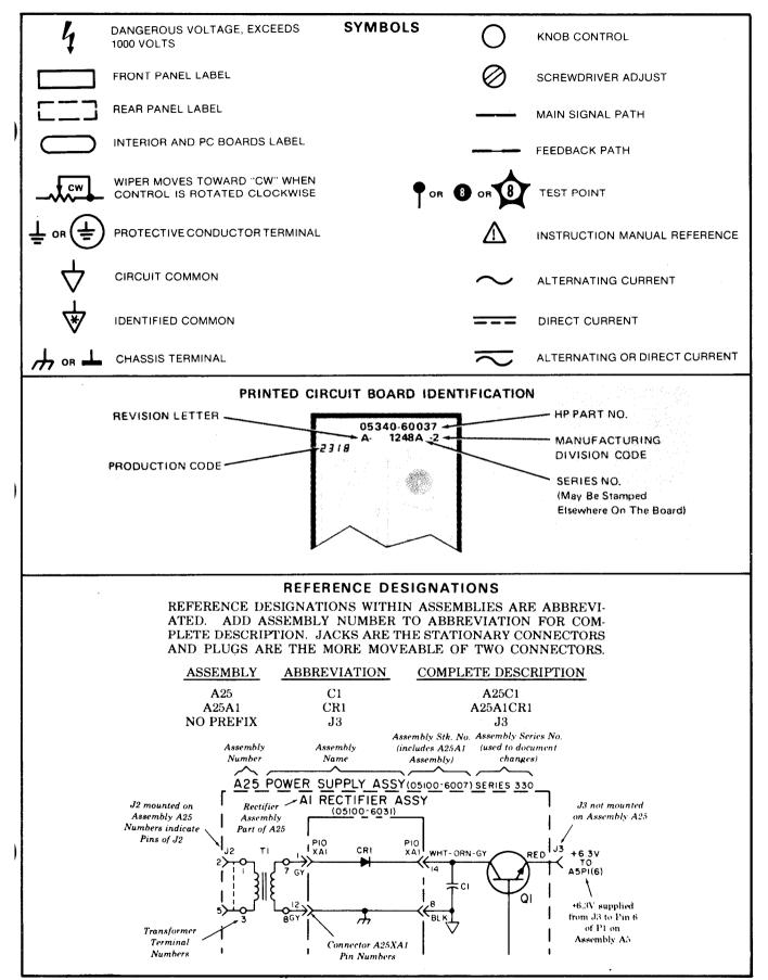
Figure 8-1. Schematic Diagrams Notes
