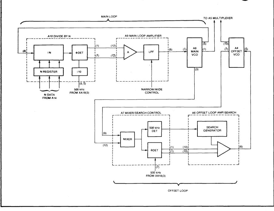
Figure 8-10. Block Diagram of Synthesizer Section
