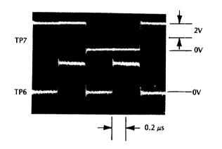
3. Check the inputs to the B counter as follows: Apply a 50 MHz, -10 dBm signal to the high frequency input and select the 500 MHz—18 GHz range. Put the 5342A in AUTO and push RESET to cause the counter to go to the prs generation, thus enabling the B counter. Place the rear panel FM switch to the FM position so that the B counter is enabled for 2.1 seconds.
