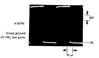
If the above waveform is not present, check the collector of A19Q1 for 300V (with respect to the test point TPG). If 300V dc is not present, suspect input rectifier A19CR1 and associated circuitry. If 300V dc is present, suspect open transistors Q1 and Q2.
