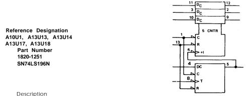
50/30 MHz PRESETTABLE DECADE COUNTER/LATCH
