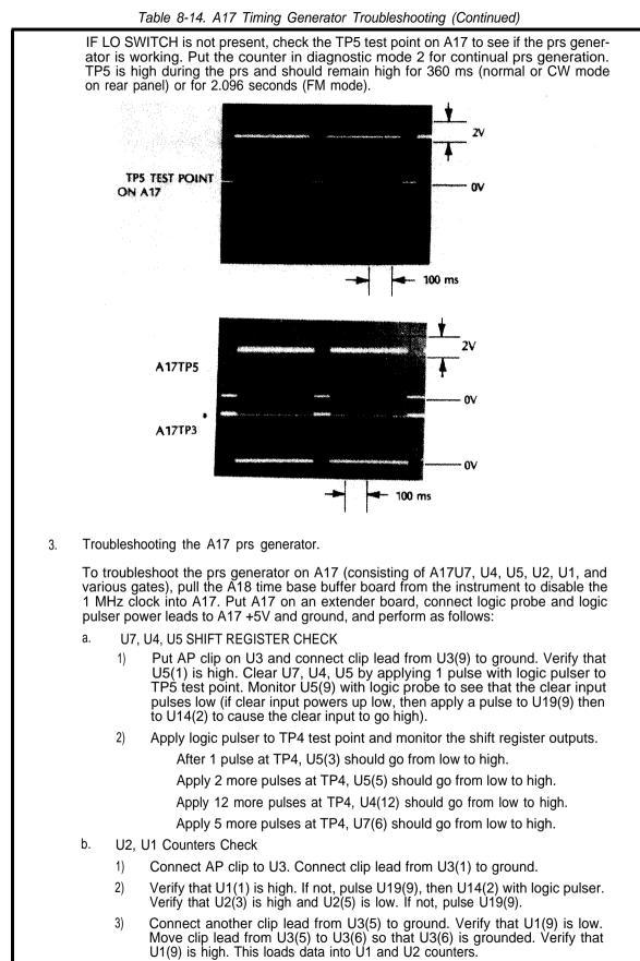
4) Monitor U1(15) with logic probe and pulse TP4 test point with pulser 14 times. ON 14th clock, U1(15) should pulse high.
