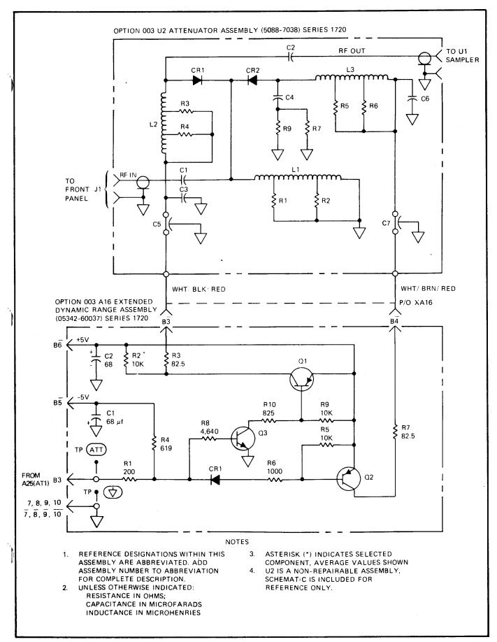
Figure 8-40. Option 003 A16 Extended Dynamic Range Assembly
