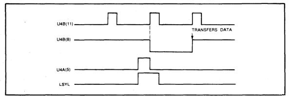
Figure 8-12. Data Transfer Timing in A10 Circuit
