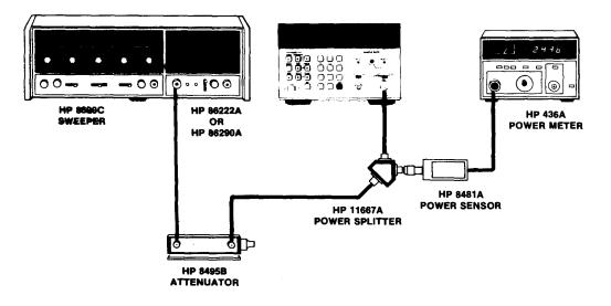
• Connect the 11667A directly to the 5342A type N connector and connect the 8481A directly to the other 11667A output.
