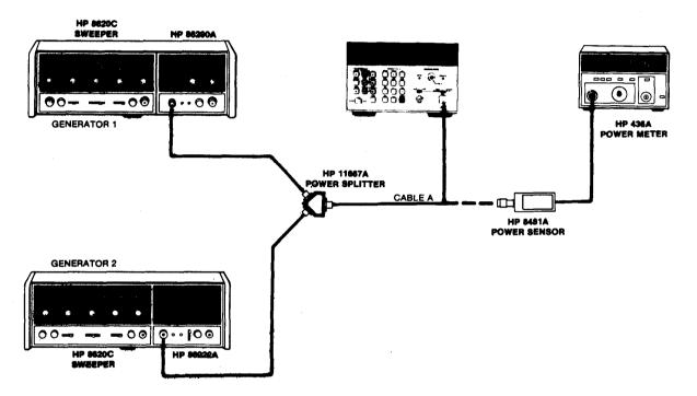
Set generator 1 to 18 GHz and at a level to deliver -5 dBm to the 5342A. To set this level, disconnect generator 2 from the 11667A and terminate that input port of the 11667A with a 909A (Option 012)  $50\Omega$  termination. Connect the 8481A to the 5342A end of cable A and adjust the 86290A output fer a -5 dBm reading.
