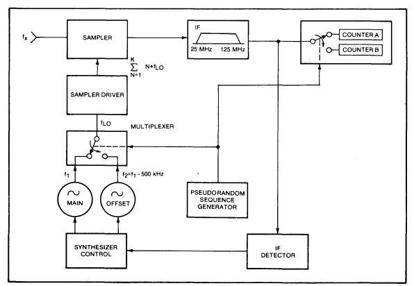
Figure 8-8. HP 5342A Simplified Block Diagram
