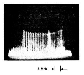
e. If the spectrum analyzer display remains as in the first photo, or if the IF is centered as shown below, then change A9R16 to 15  $M\Omega$  (0683-1565).
