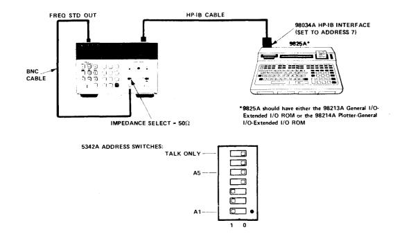
4-21. To perform the verification, set up the 5342A as shown and set its rear panel address switches to address 07.
