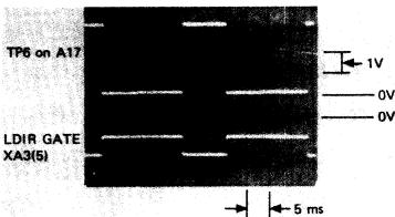
As the resolution is changed, the width of the gate signal (TP6 high) should vary as follows:
