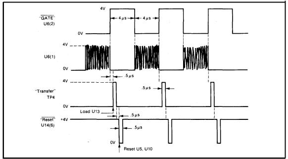
Figure 8-13. Filter Timing on A12 IF Detector
