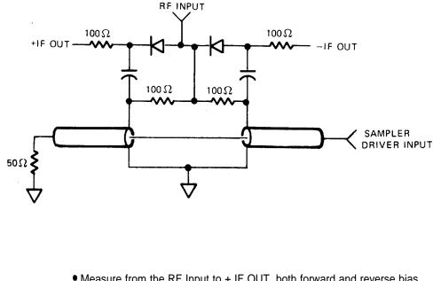
• Measure from the RF Input to + IF OUT, both forward and reverse bias.
