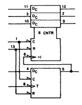
Description 30 MHz PRESETTABLE BINARY COUNTERS/LATCHES
