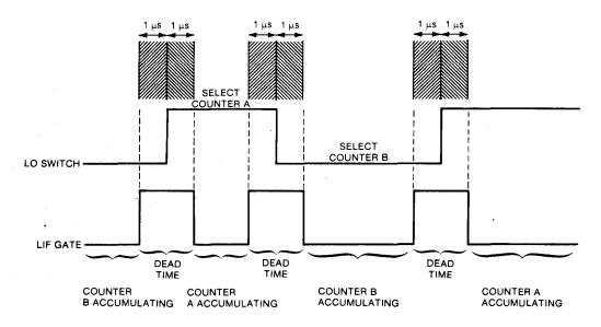
8-254. The dead time in the LIF GATE signal is generated by D flip-flops U9A, U9B, exclusive "OR" U6D, and D flip-flop U15A. The dead time is generated when U6D(11) goes high for two periods of the 1 MHz clock. With U6D(11), high, U10B is disabled and the prs clock at U10C(8) remains high. The reset input to U15A(1) is low during the prs generation so that U15A(5) is low. When the preset input U15A(4) goes low also, the output goes high for the time that the preset
