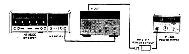
a. Set 8620C to 75 MHz at -15 dBm. Ihile monitoring the rear panel IF OUT power with the 436A Power Meter, adjust A25R28 "BAL" for maximum signal level as read on the 436A.
