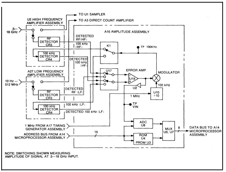
8-17. Option 002 Amplitude Measurements Block Diagram
