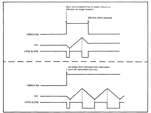
Figure 8-11. Timing Diagram or A6 Search Generator Operation
