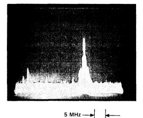
d. Reduce input signal level until counter no longer counts 18 GHz but displays all zeros. The IF OUT on the spectrum analyzer should appear as:
