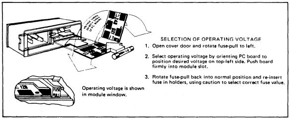
Figure 2-1. Line Voltage Selection
