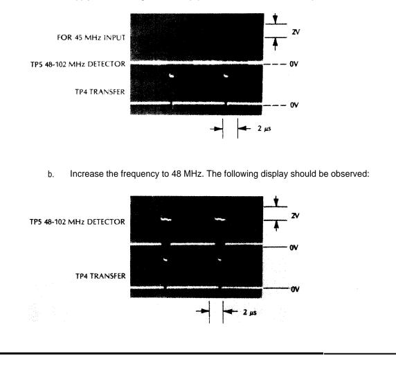
a. Apply a 45 MHz signal at 0.6V p-p to the 500 MHz—18 GHz input of the 5342A.
