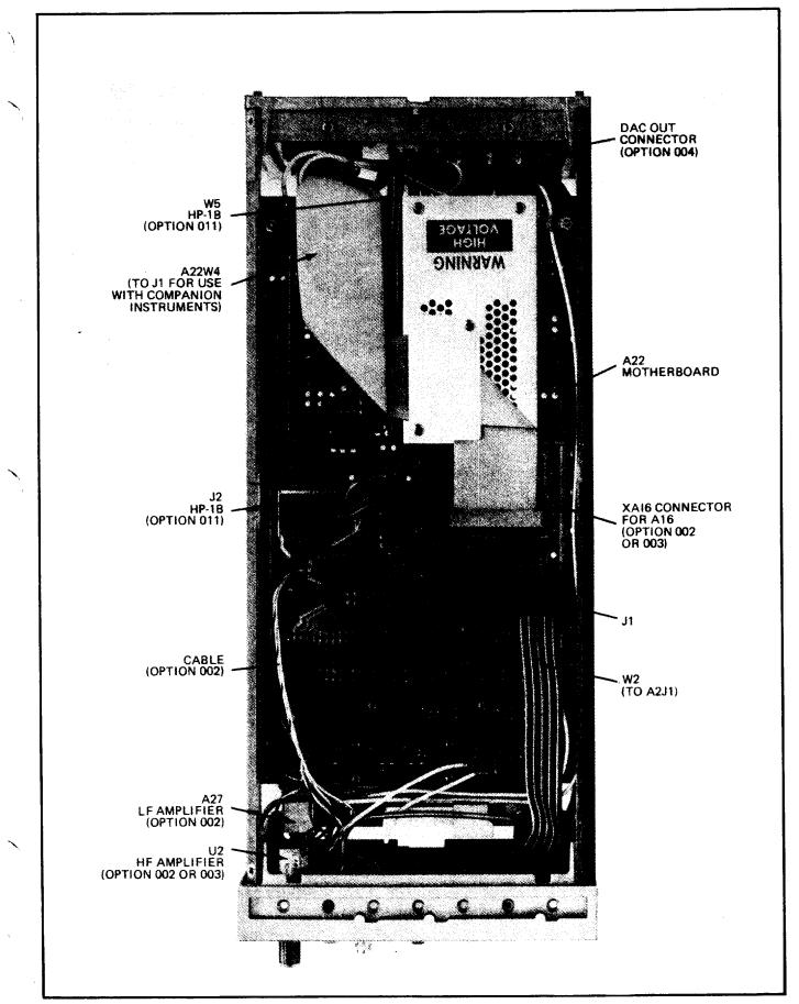
Figure 8-22. 5342A Bottom View, Options Installed
