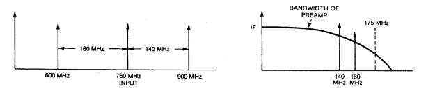
8-109. By limiting the IF to frequencies less than 125 MHz, the problem described in paragraph 8-108 does not occur. For the case of a 725 MHz input, the second harmonic of 300 MHz produces an IF of 125 MHz (the maximum allowable IF) and the third harmonic produces an IF of 175 MHz. But the IF signal at 175 MHz is attenuated by the175 MHz bandwidth of the preamplifier as shown below so as to prevent errors in counting.
