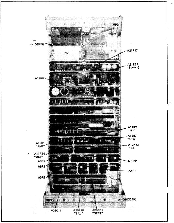
Figure 8-21. 5342A Top View (Assembly Locations and Adjustments)
