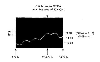
FOR AMPLITUDE OPTION, put the 5342A in diagnostic **mode** 5 (press SET, SET 5) to prevent switching between the sampler input and the peak detector input. Measure SIR as described above and verify that for amplitude measurements, return loss is >9.5 dB for frequencies from 2 GHz-18 GHz. Next put the 5342A in AUTO and frequency only so that amplitude measurements are not made. Verify that the return loss is >3.5 dB for frequencies from 2-18 GHz (SIR <5:1).
