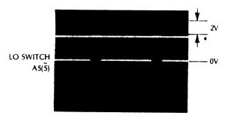
The time during which the signal switches between high and low levels in a pseudorandom fashion should be 360 ms. The time where the signal is high and not switching is controlled by the front panel sample rate control and resolution of counter. If the rear panel switch is placed in the FM position, then the time during which the signal is switching should extend to 2.1 seconds (actually 2.096).
