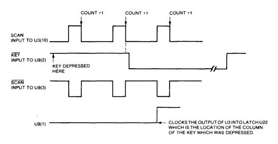
8-140. With KEY low and SCAN low, U9(1) goes high which clocks latch U22 and causes it to store the address (0000 to 1100) of the column of the key which was pushed. Since there are two keys per column, another line is used to indicate top or bottom row, The output of U9(1), which clocks U22, also clocks U19A. U19A(5) will be low if a top row key is pushed and will be high if a bottom row key is pushed. In this manner, the microprocessor determines exactly which key has been depressed.
