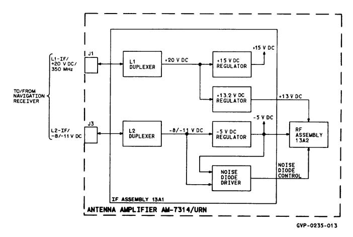
FIGURE 3-6. Antenna Amplifier AM-7314/URN, Power Distribution and Control
