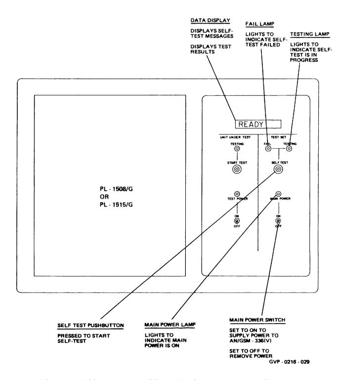
FIGURE 6-2. AN/GSM-336(V)2 or AN/GSM-336(V)3, Controls and Indicators (Sheet 1 of 2)
