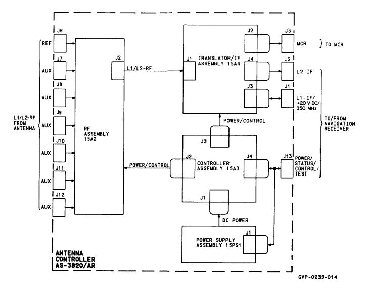
FIGURE 3-11. Antenna Controller AS-3820/AR, Block Diagram
