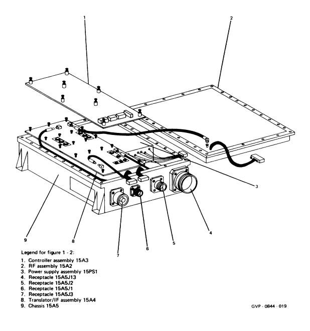
FIGURE 1-2. Antenna Controller AS-3820/AR, Reference Designations
