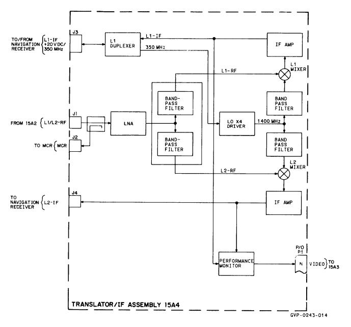
FIGURE 3-17. AS-3820/AR Translator/IF Assembly 15A4, Block Diagram
