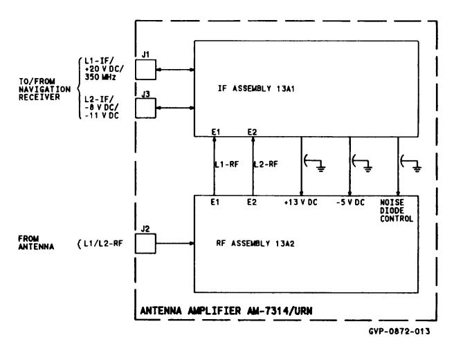
FIGURE 3-7. Antenna Amplifier AM-7314/URN, Interconnect Wiring Diagram
