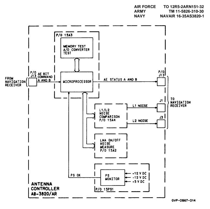
FIGURE 3-18. AS-3820/AR Built-in Test, Functional Diagram
