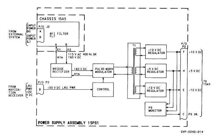
FIGURE 3-14. AS-3820/AR Power Supply Assembly 15PS1, Block Diagram
