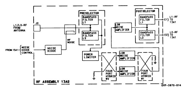
FIGURE 3-9. AM-7314/URN RF Assembly 13A2, Block Diagram
