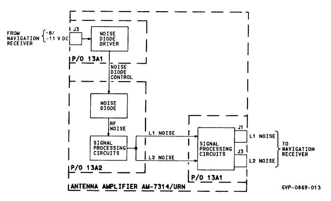
FIGURE 3-10. AM-7314/URN Self-Test, Functional Diagram
