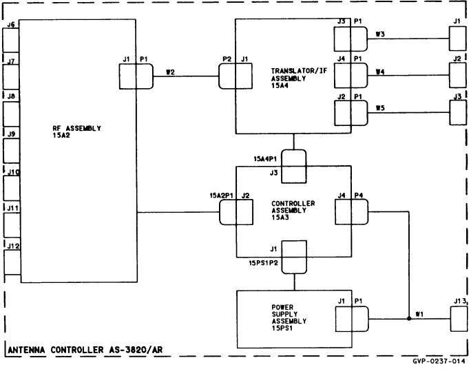
FIGURE 3-13. Antenna Controller AS-3820/AR, Interconnect Wiring Diagram
