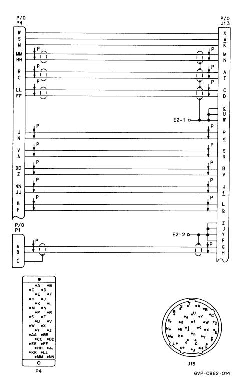
FIGURE 6-1.AS-3820/AR, Wiring Diagram
