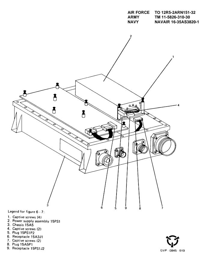
FIGURE 6-7.AS-3820/AR Power Supply Assembly 15PS1, Removal/Installation
