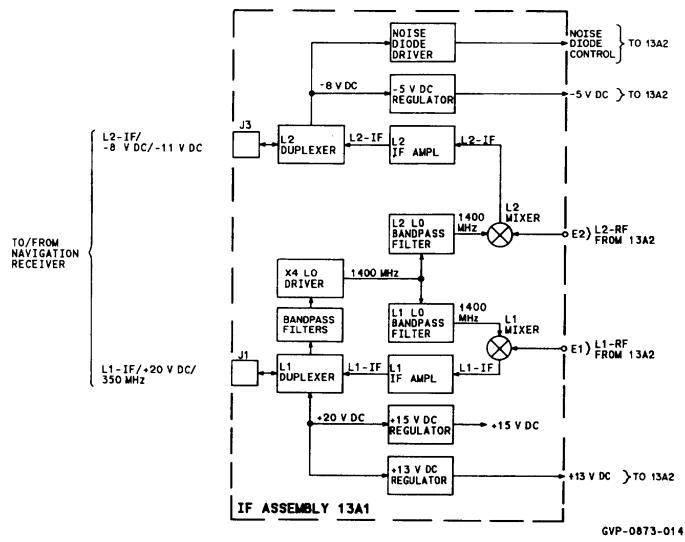
FIGURE 3-8. AM-7314/URN IF Assembly 13A 1, Block Diagram
