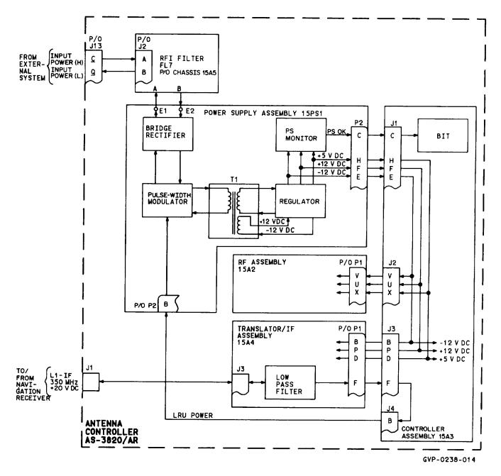
FIGURE 3-12. Antenna Controller AS-3820/AR, Power Distribution and Control
