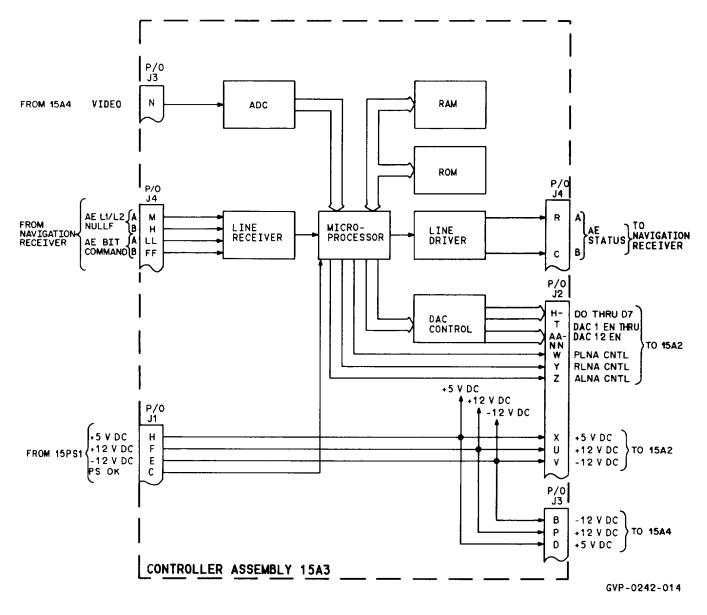
FIGURE 3-16. AS-3820/AR Controller Assembly 15A3, Block Diagram
