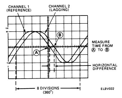
14. Determine horizontal difference between corresponding points on waveforms at common horizontal graticule line and calculate phase difference using formula:
