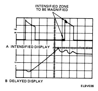
11. Calculate apparent sweep magnification using formula:
