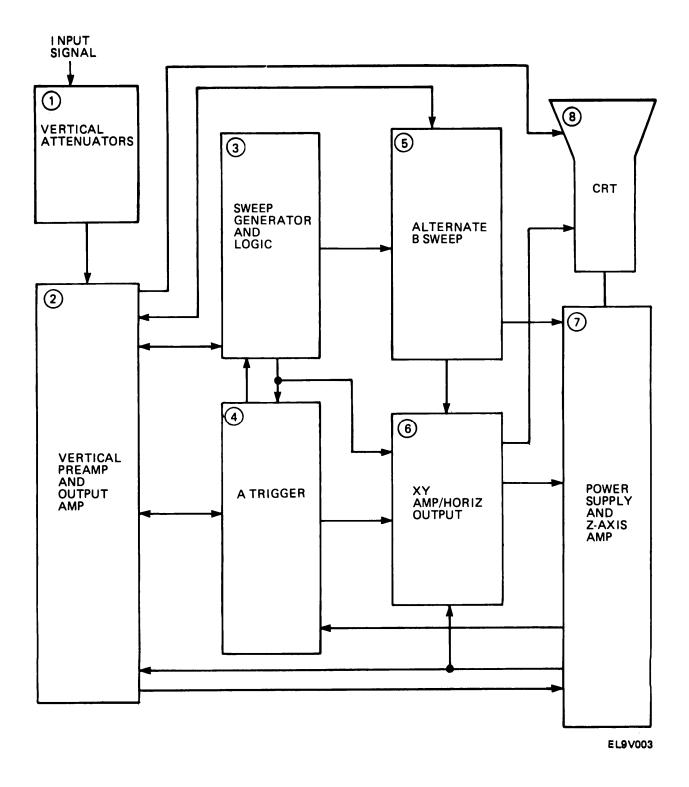
Figure 1-2. AN/USM-488 Oscilloscope Block Diagram
