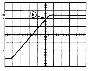
THE 10% POINT ON THE WAVEFORM INTERSECTS THE 90% POINT ON THE WAVEFORM INTERSECTS THE CENTER VERTICAL GRATICULE LINE.
