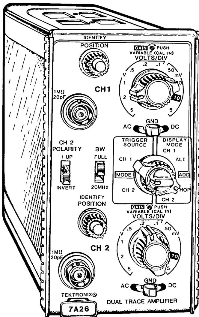
Fig. 1-1. AM-6785A/U 7A26 Dual Trace Amplifier.
