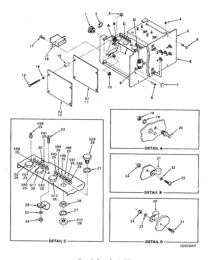
Figure 7. Power Supply (A1)
