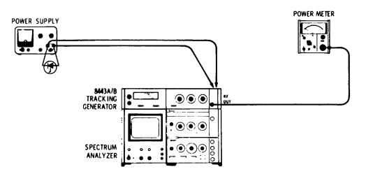
Figure 5-5. ALC/Video Amplifer Test Setup
