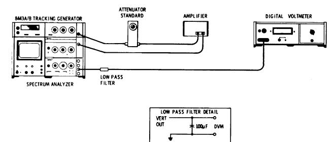
Figure 4-2. Amplitude Range Test Setup
