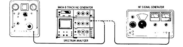
Figure 4-1. Frequency Range Test
