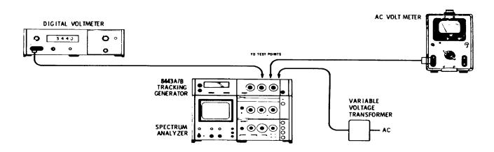
Figure 5-1. Power Supply Test Setup
