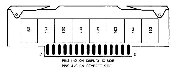
Figure 8-38B. A1A2, Counter Display Board Assembly, Components (CHANGE 9)
