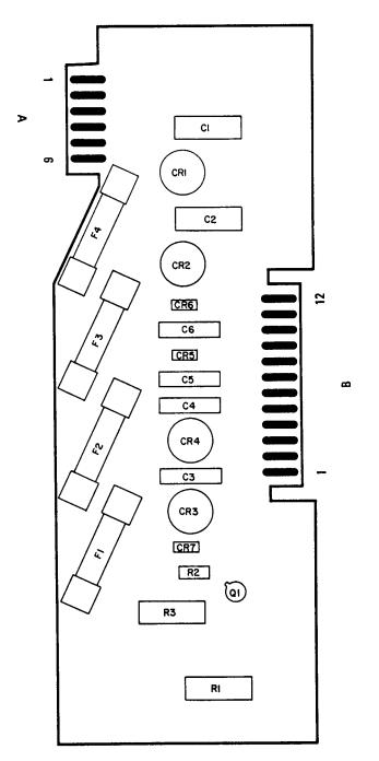
Figure 8-29. A15, Rectifier Assembly, Components (CHANGE 12)
