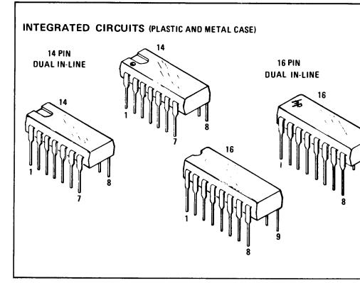
Figure 8-16. Integrated Circuit Packing
