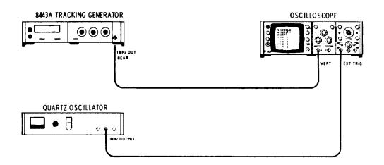
Figure 5-6. Reference Oscillator Test Setup
