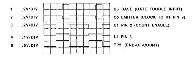
Figure SS8-3. Gate Toggle, Count Enable, and End-of-Count Waveforms (CHANGE 10)
