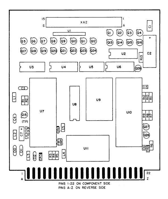
Figure 8-38A. A1A1, Low Frequency Counter Board Assembly, Components (CHANGE 9)
