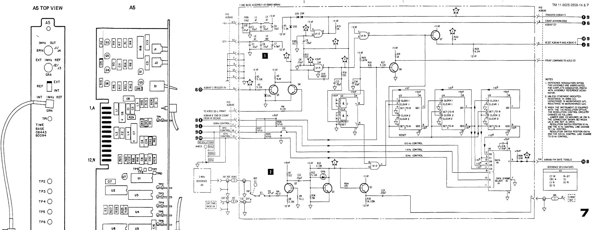
Figure 8-34. A5 Time Base Assembly, Cover and Components (CHANGE 13)
