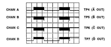
Figure SS84. Output Waveforms, MARKER Mode (CHANGE 10)
