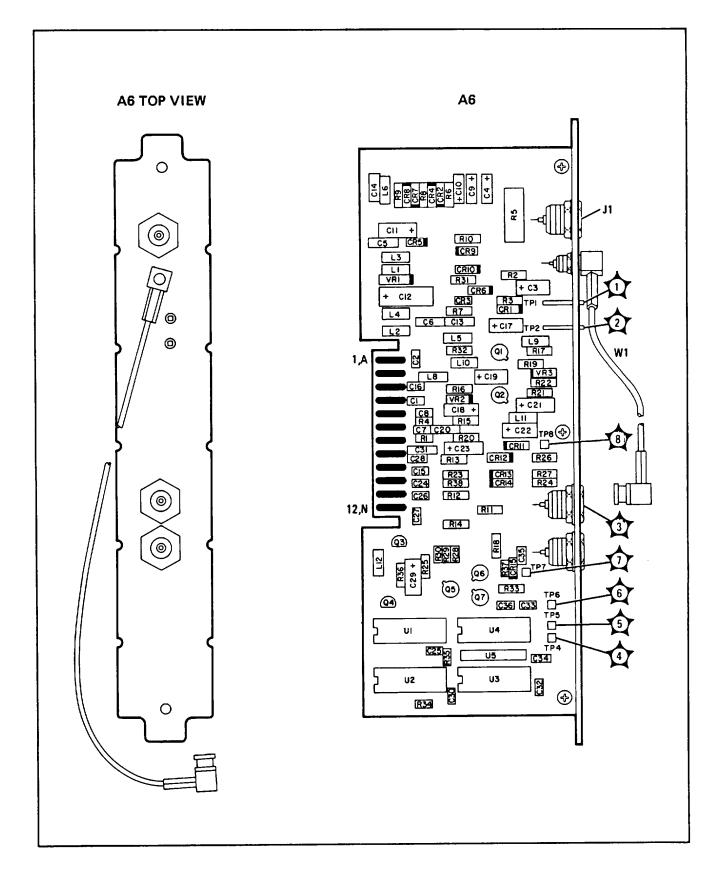
Figure 8-36. A6, High Frequency Decade Assembly, Cover and Components (CHANGE 10)
