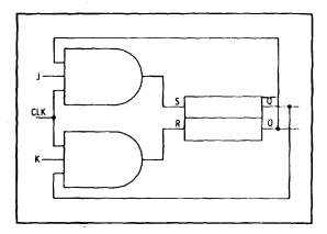
Figure 8-9. Clocked JK Flip-Flop
