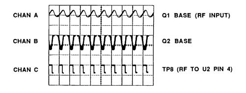
Figure SS8-2. RF Amplifier Waveforms (CHANGE 10)
