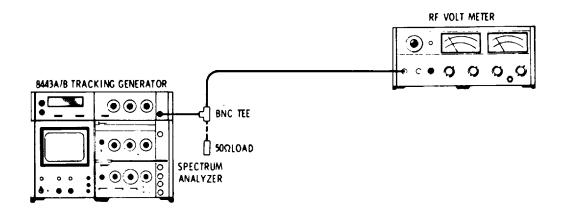
Figure 4-4. Output Impedance Test Setup
