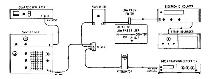
Figure 4-5. Time Base Again Rate Test
