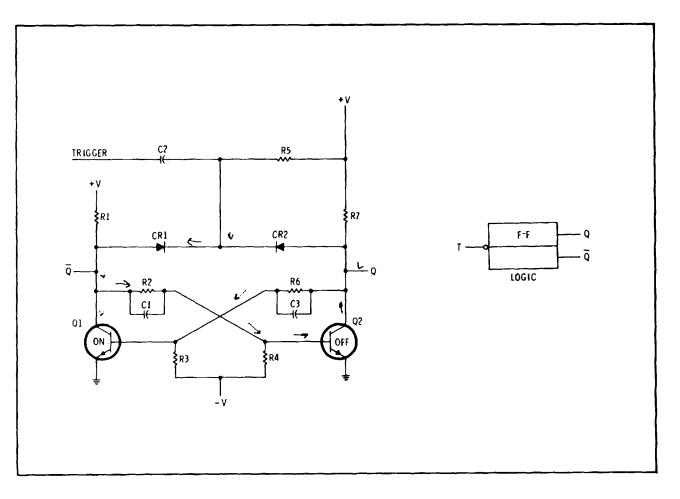
Figure 8-6. Triggered Flip-Flop
