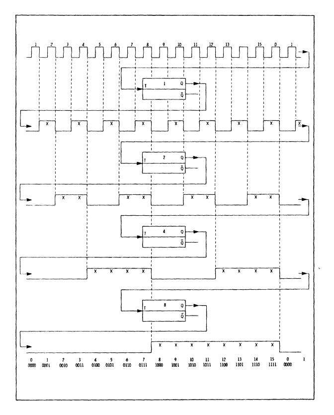
Figure 8-11. 16 Counter Binary Counter Chain
