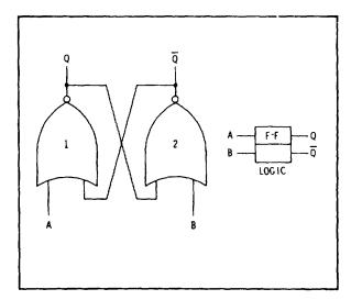
Figure 8-5. Basic NOR Gate Flip-Flop
