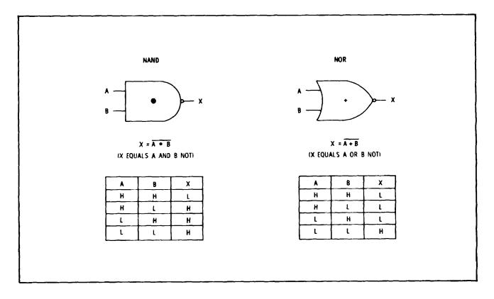
Figure 8-3. Basic NAND and NOR Gates
