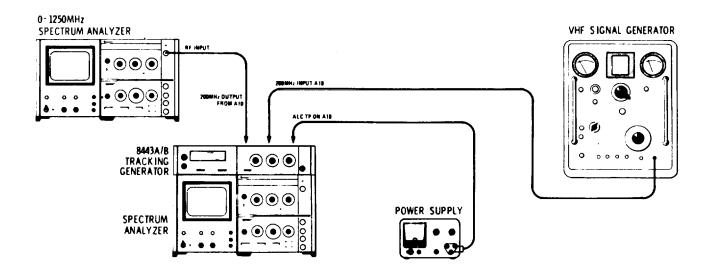
Figure 5-3. 200 MHz IF Test Setup
