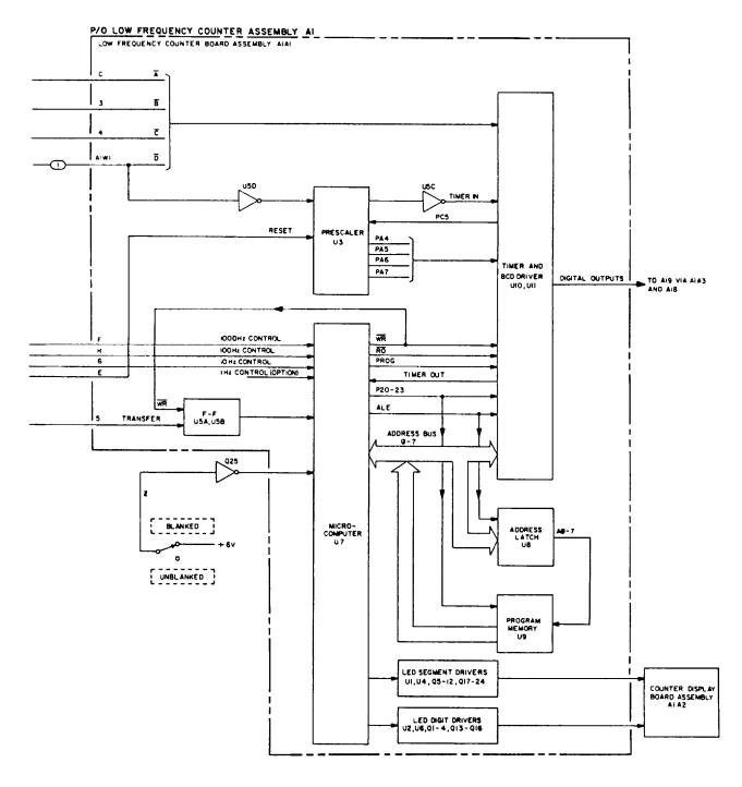
P/O Figure 8-31. Counter Section Logic Diagram (Low Frequency Counter Portion) (CHANGE 9)
