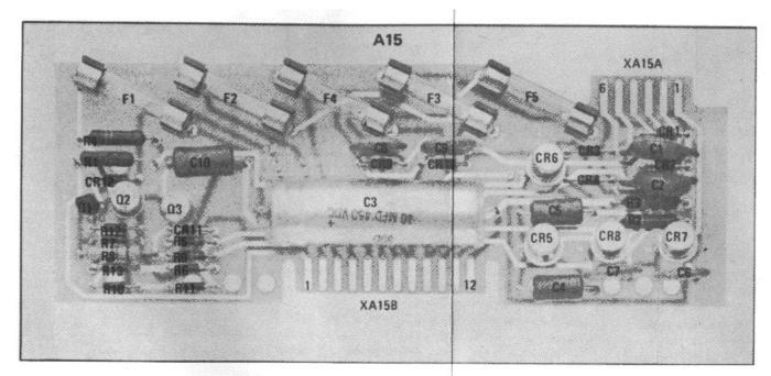
Figure 8-29. A15, Rectifier Assembly, Components
