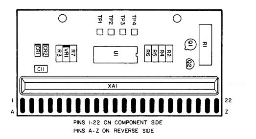
Figure 8-38C. A1A3, +6V Switched Board Assembly, Components (CHANGE 9)
