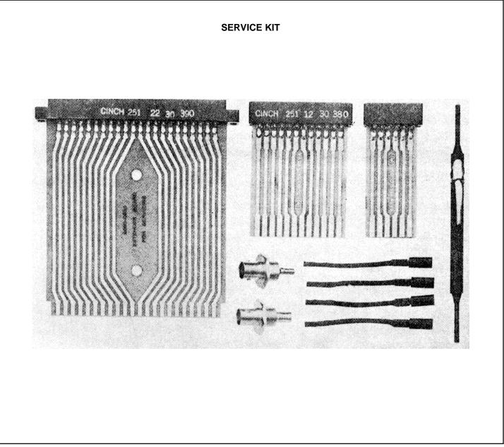
Figure 1-3. Service Kit Required for Maintenance
