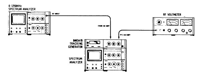
Figure 5-4. Third Converter Test Setup
