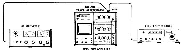
Figure 5-2. First Converter Test Setup
