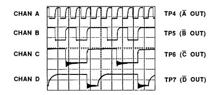
Figure SS8-1. Output Waveforms, SCAN HOLD Mode (CHANGE 10)
