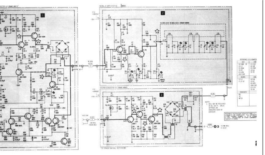
Figure 8-23. First and Second Converter and IF Amplifier, Schematic Diagram
