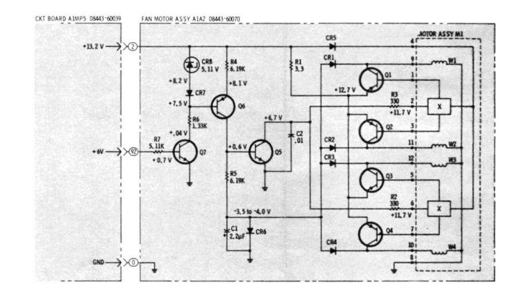
Figure 8-42. Fan Motor Credits, Schematic Diagram
