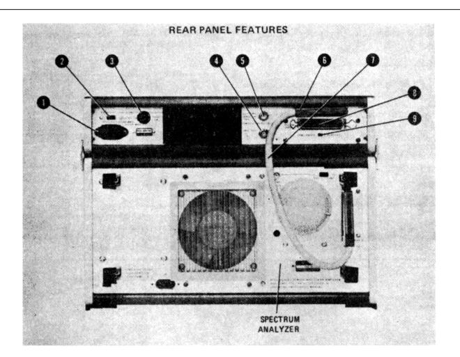
(1) LINE Power Jack: connection for line power cable.
