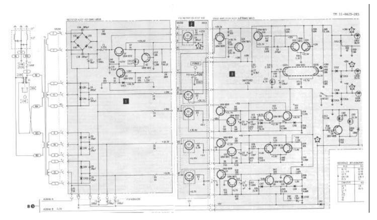
Figure 8-30. Power Supplies and Regulators, Schematic Diagram
