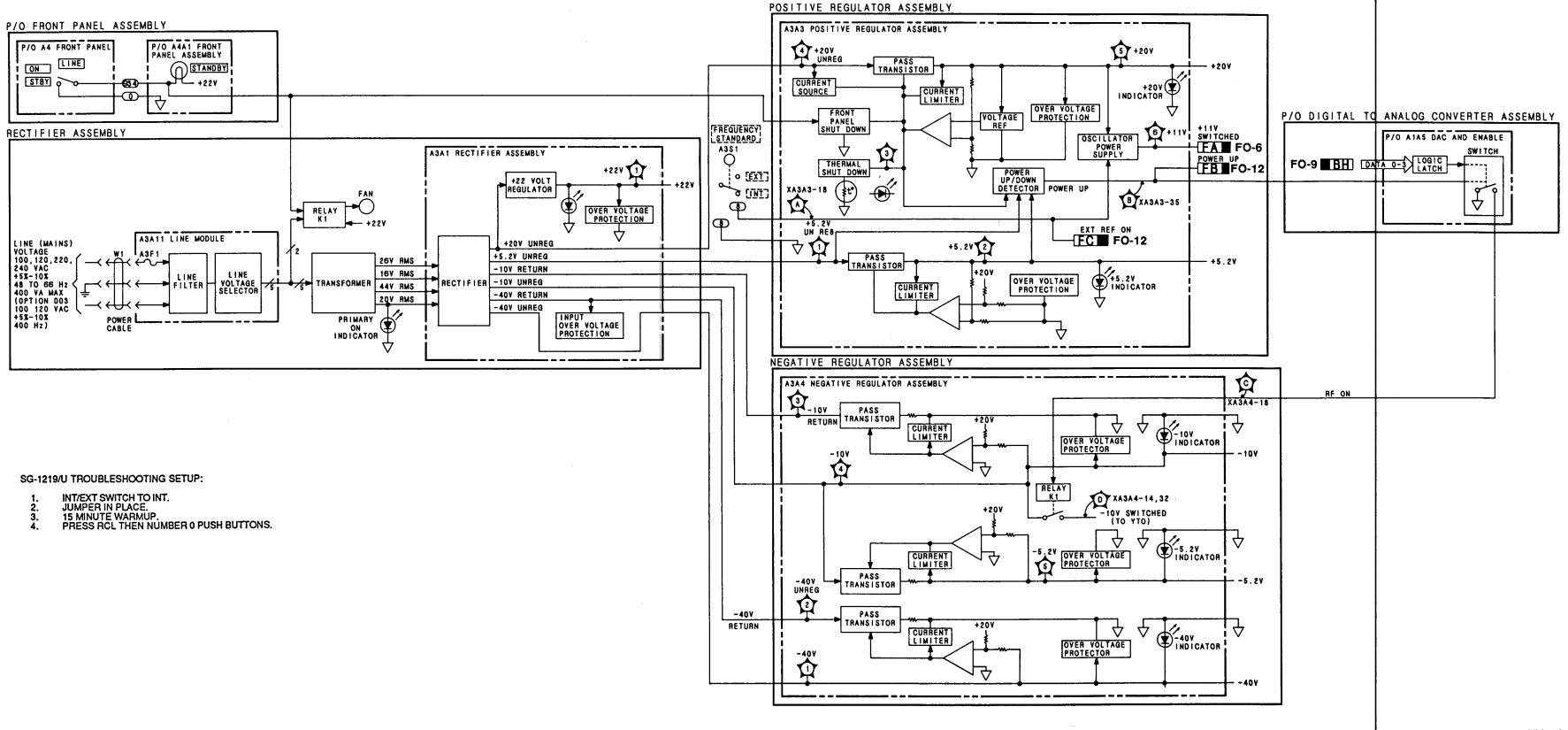
Figure FO-13. Power Supply Subsystem Functional Block Diagram.
