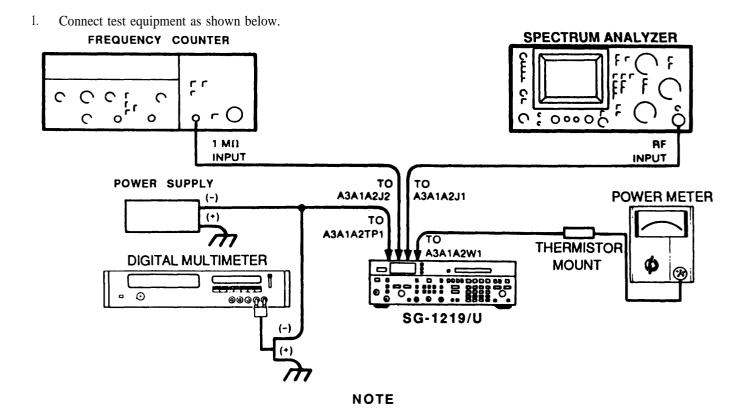
Connect Frequency Counter to A3A1A2J2 (fig. FO-4) in place of termination and connect Spectrum Analyzer to A3A1A2J1 in place of A3A1A1W1 (gray/orange/white).
