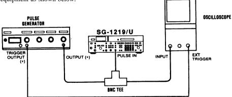
13. Set Pulse Generator for 1 pulse per microsecond (1 MHz PRF) and a pulse width of 200ns.
