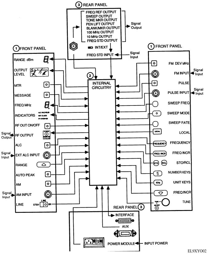
Figure 1-2. Signal Generator Block Diagram.
