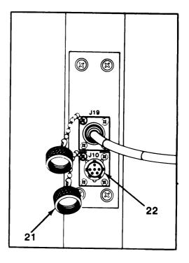
11. Aline df cable connector J10 keys to connector J10 (23) on antenna mast column (24).
