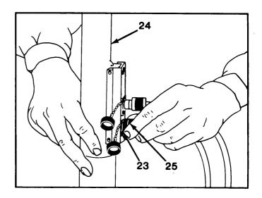
12. Push in on cable collar (25) and turn clockwise to screw in place.
