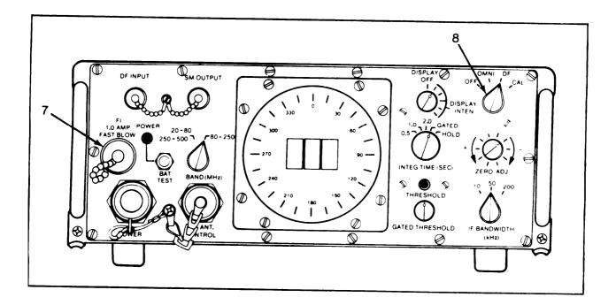
**NOTE** Return to the troubleshooting table after removing and replacing the df processor fuse. Troubleshooting procedures must be completed.
