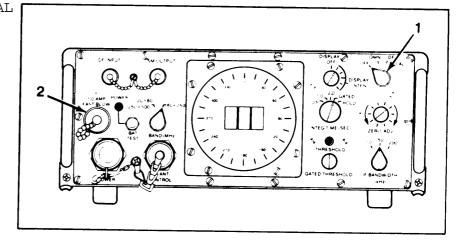
3. push in on 1.0 AMP FAST BLOW cap (3) on front panel and turn 1/4 turn counterclockwise.
