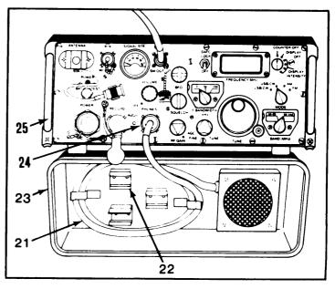
13. Remove protective cap from RF INPUT (26) on receiver (25) by pushing in and turning 1/4 turn counterclockwise.
