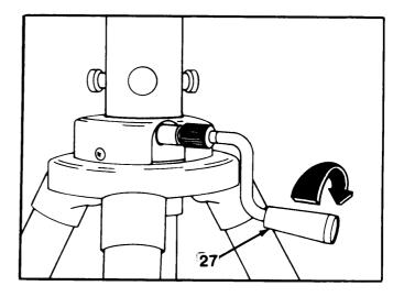
20. Holding crank handle (27), handtighten COLUMN LOCK knob (28) by turning clockwise.
