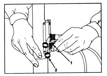
DISCONNECTING DF ANTENNA CABLES (SHEET 2 OF 3)
