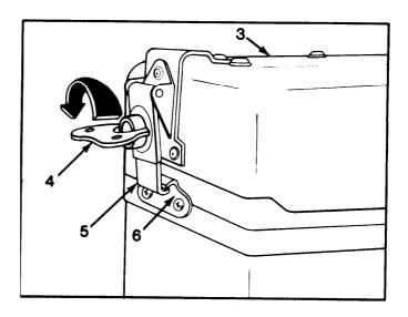
BA-4386/PRC-25 BATTERY PACK INSTALLATION (SHEET 2 OF 3)
