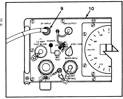
6. Remove protective cap from SM OUTPUT (11) on df Processor (10) by pushing in and turning 1/4 turn counterclockwise.
