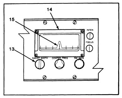
13. Rotate SM GAIN knob (16) clockwise until a baseline of small noise spikes (17) appear on the signal monitor screen (14).
