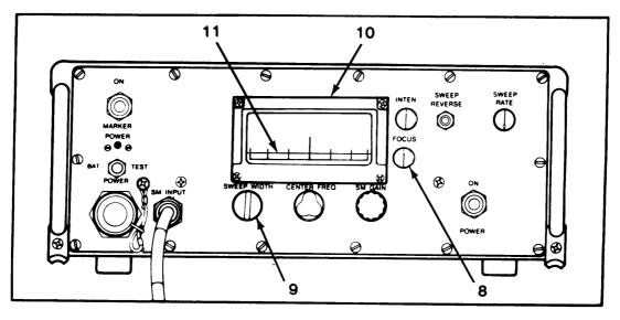
10. Rotate CENTER FREQ knob (12) until line (11) on signal monitor screen (10) reaches maximum height.
