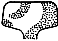
Fig. B Compound Fissure
