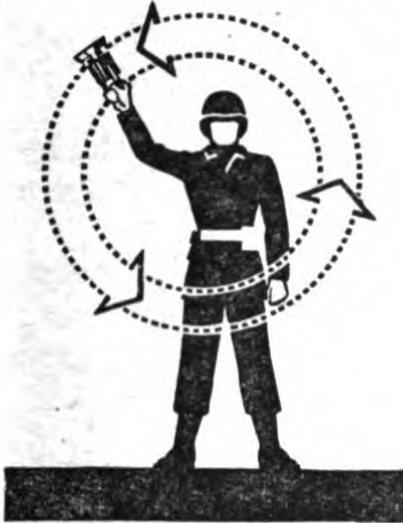
Figure 5. TRAIN HAS PARTED. Lamp swung vertically in a circle at arm's length across the track.
