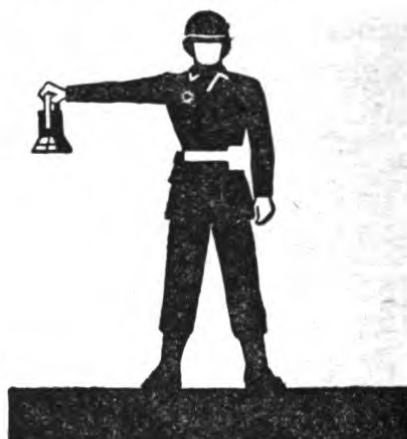
Figure 2. REDUCE SPEED. Lamp held horizontally at arm's length.
