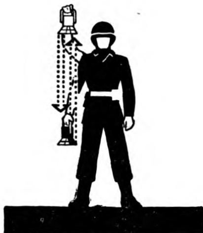
Figure 3. PROCEED. Lamp raised and lowered vertically.
