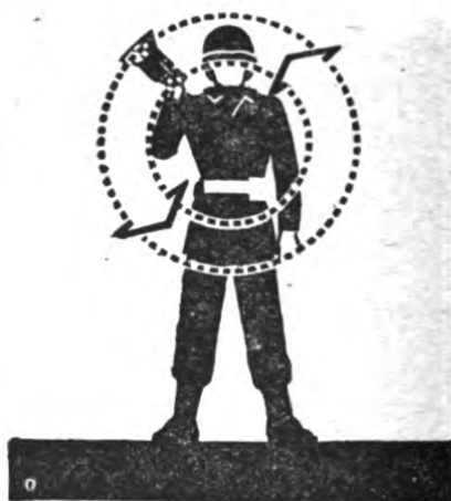
Figure 4. BACK. Lamp swung vertically in a circle at half arm's length across the track.
