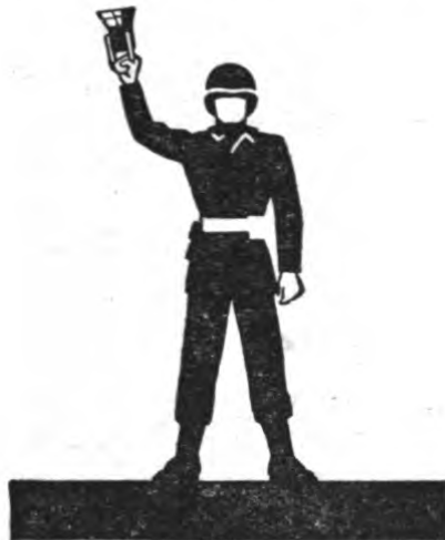
Figure 7. RELEASE AIR BRAKES. Lamp held at arm's length above the head when standing.
