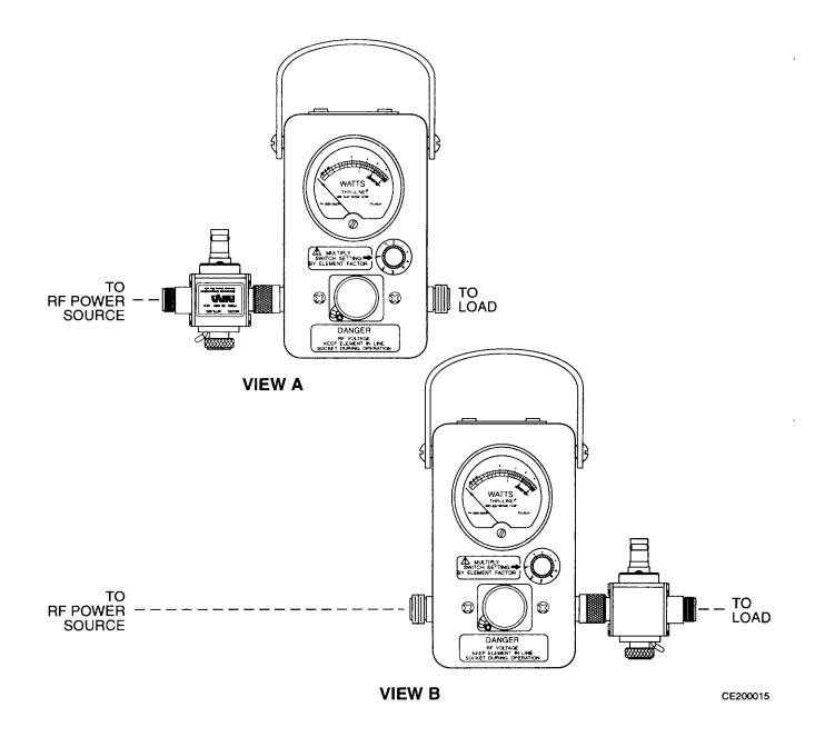
• If a load match measurement is to be taken, connect RF test set as shown in View A.
