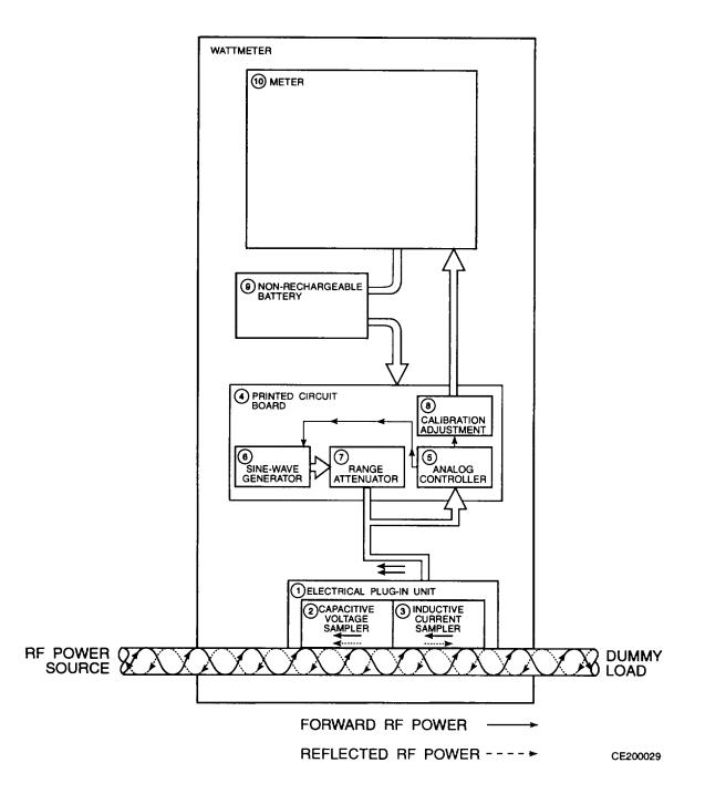
Figure 5-2. Wattmeter Functional Block Diagram
