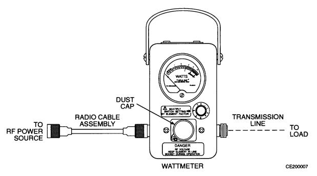
c. Select an electrical plug-in unit with a range that includes the frequency and power level of the RF power source being tested.
