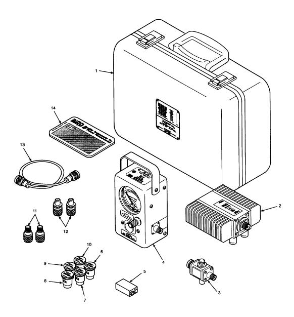
Figure F-1. Radio Frequency Power Test Set AN/URM-213
