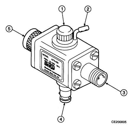
Figure 2-2. Operator's Controls, Indicators, and Connectors - Coupler
