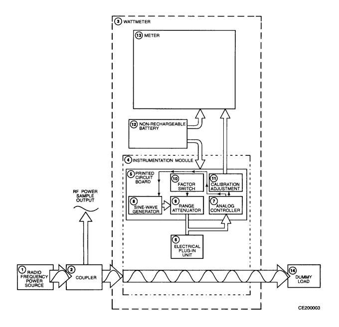
Figure 1-2. Radio Frequency Power Test Set AN/URM-213 Simplified Block Diagram
