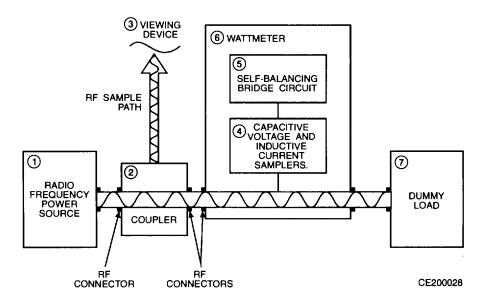
Figure 5-1. RF Test Set Functional Block Diagram
