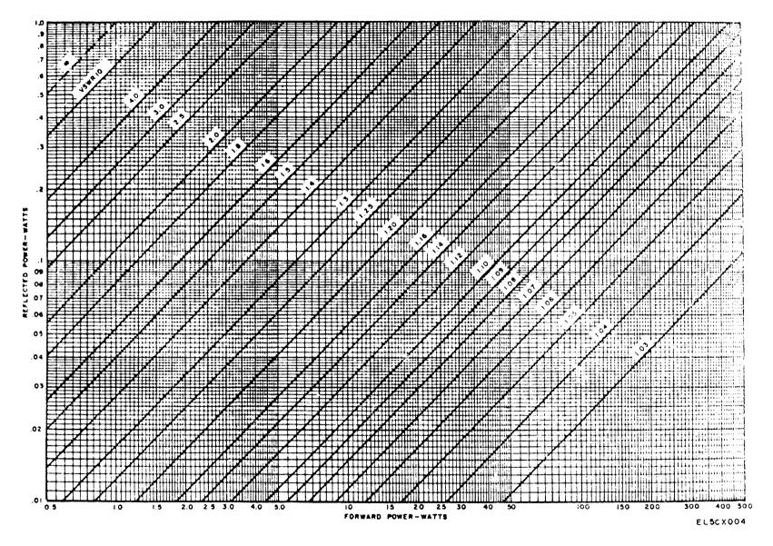
Figure 3-2. Power values versus VSWR (reflected power 0.01 to 1.0 watts).
