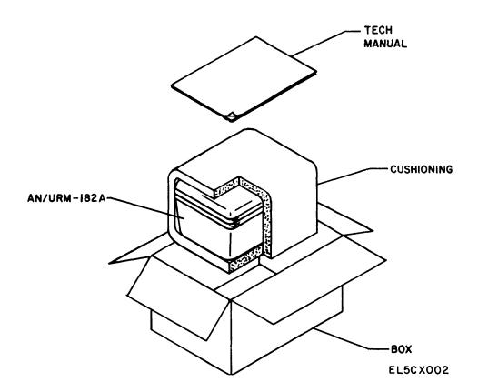
Figure 2-1. Equipment packing and packaging
