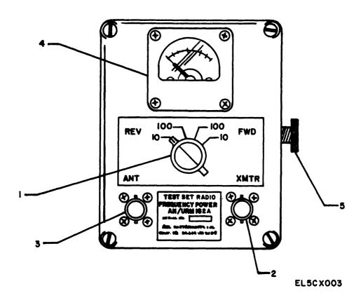
Figure 3-1. Operator's contols, indicator, and connectors.
