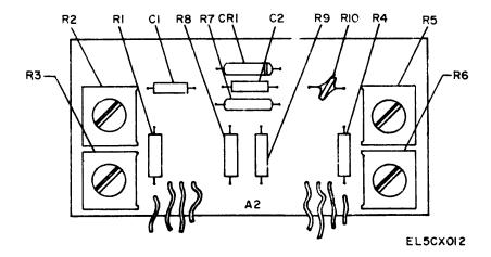
Figure 8-5. TS-3754/U, A2 printed circuit boar, parts location.
