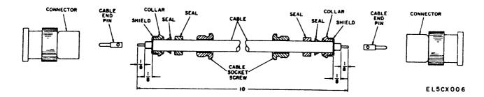
Figure 5-1. Cable assembly CG-1893/U, fabrication diagram.
