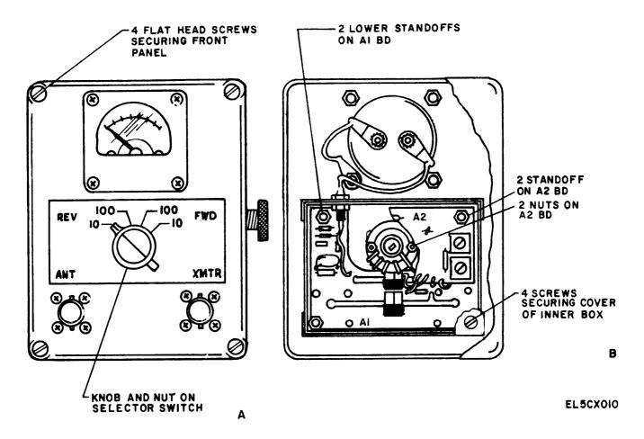
Figure 8-3. TS-3754/U, chassis parts location diagram.
