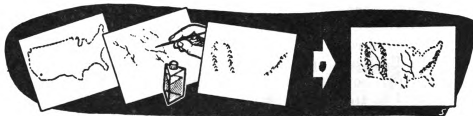
Figure 20. Preparation of transparency by using sepia lithofoil intermediates.
