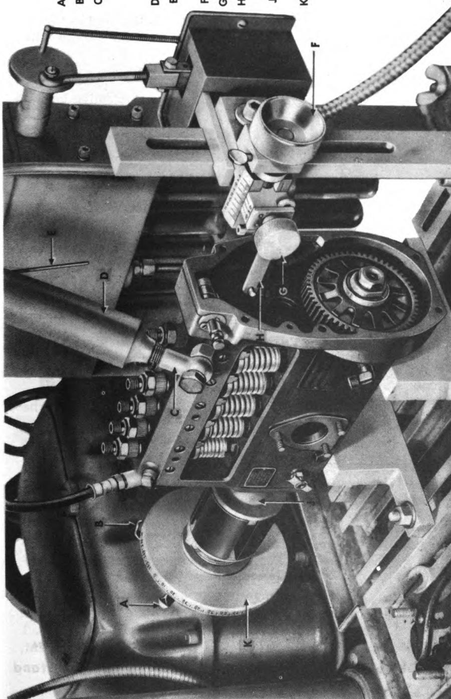
**Figure 114—Set-up for Timing Fuel Injector Pump**
