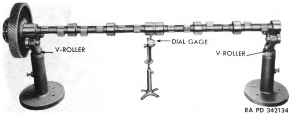
Figure 31—Checking Camshaft Alinement
