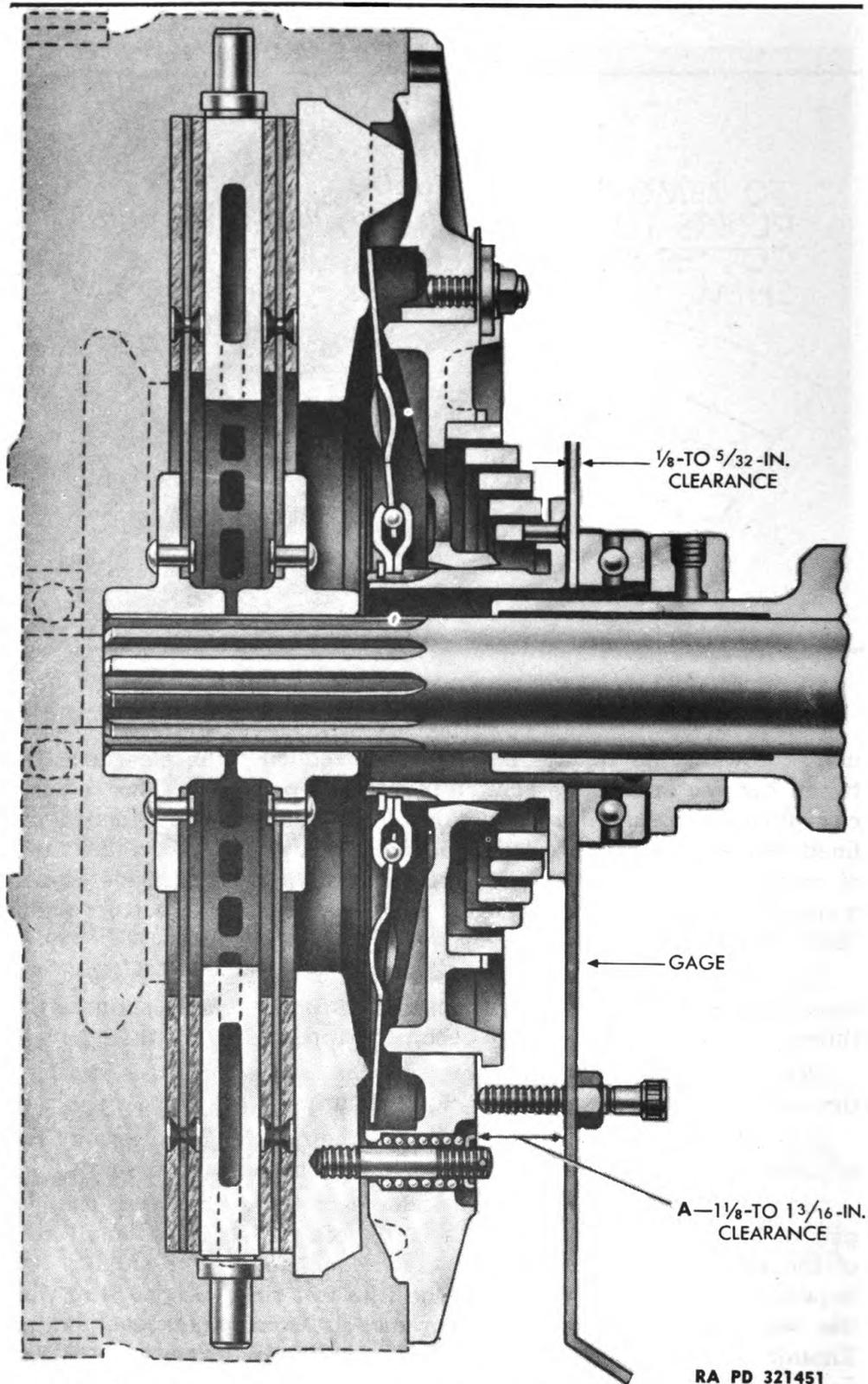
Figure 105—Cross Section, Showing Shim Adjustment of Clutch
