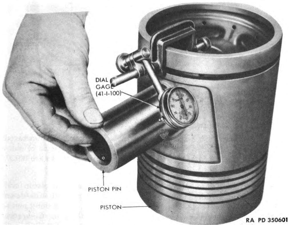
Figure 43—Checking Clearance of Piston Pin in Piston
