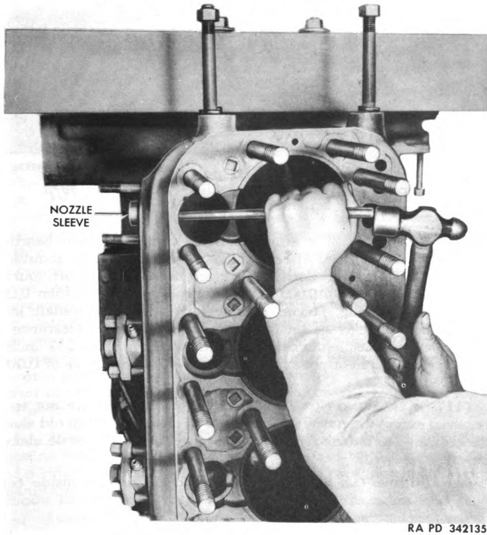
Figure 32—Removing Nozzle Sleeve, Using Steel Bar 1/2 inch in Diameter
