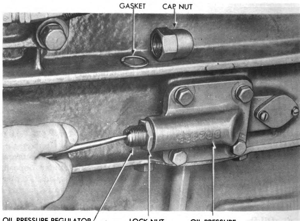
OIL PRESSURE REGULATOR VALVE ADJUSTING SCREW      LOCK NUT      OIL PRESSURE REGULATOR BODY
