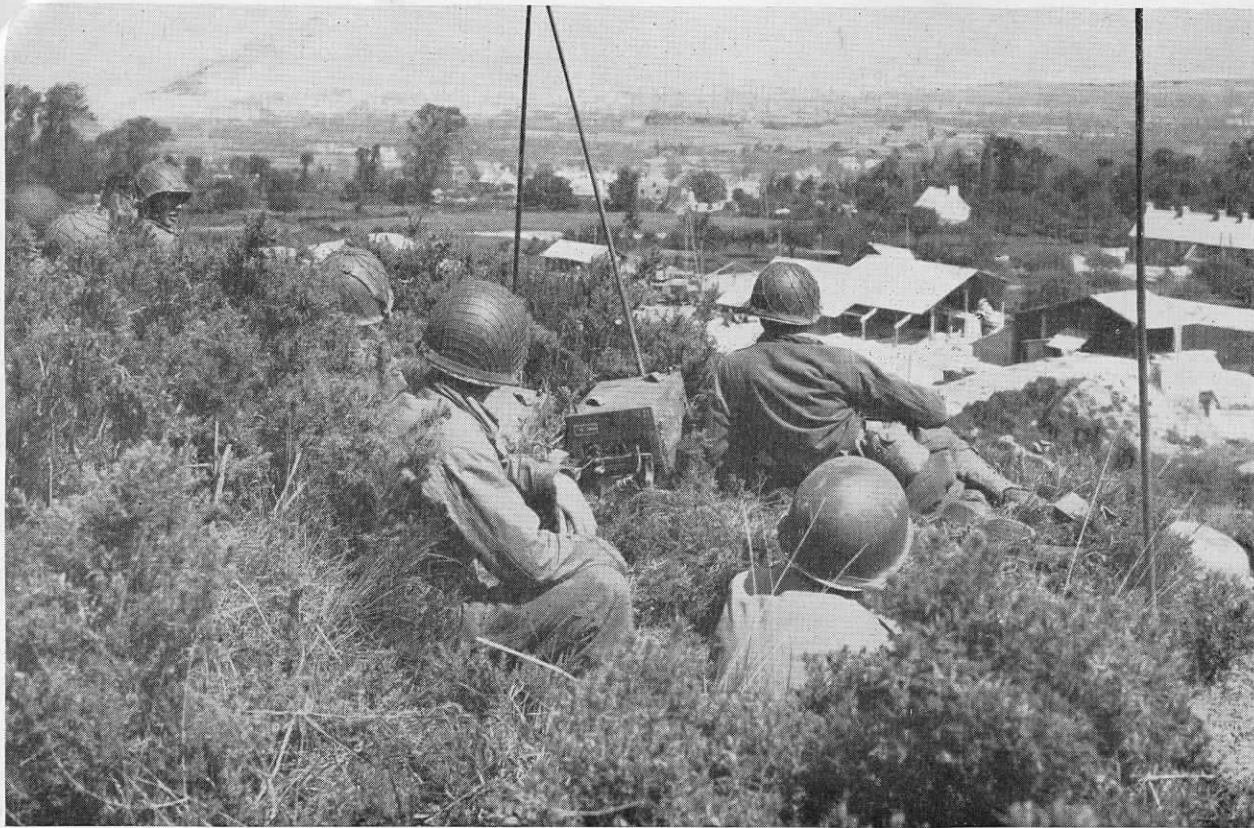
THESE SCR 608s ARE BEING USED TO RADIO BACK ARTILLERY DATA FROM AN OP OVERLOOKING THE CITY OF CHERBOURG
