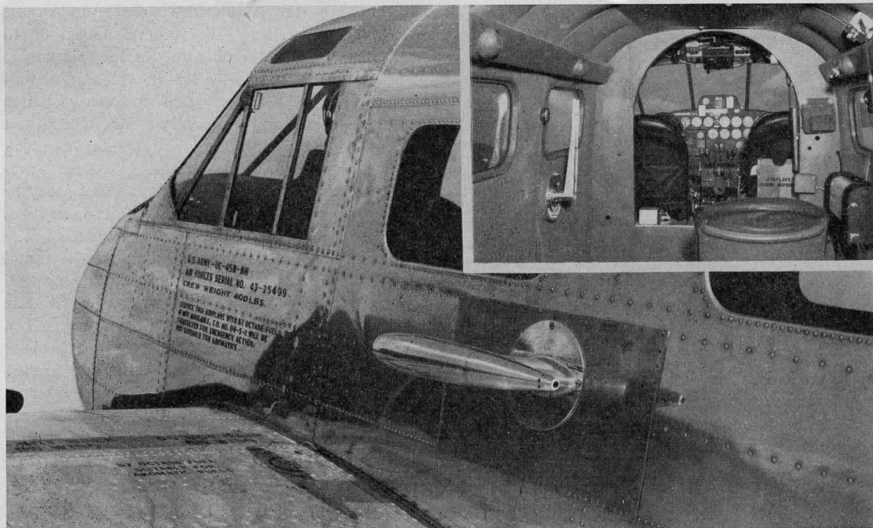
ML-313/AM VENTILATOR IN A C-45. INSERT SHOWS THE PSYCHROMETER ASSEMBLY IN THE INTERIOR OF PLANE
