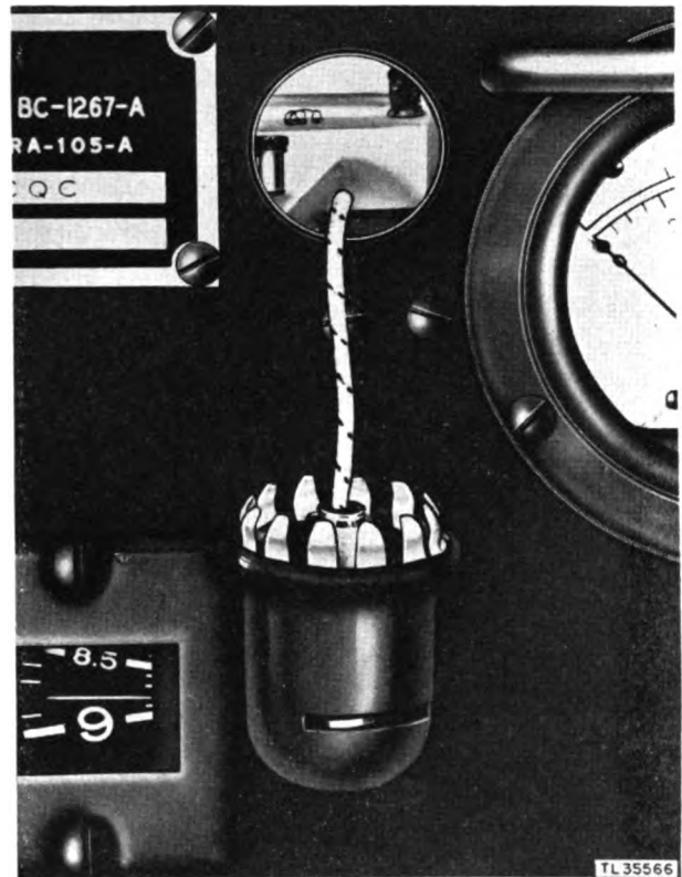
Figure 107. Radio Receiver and Transmitter BC-1267-A, meter-light housing removed from panel.
