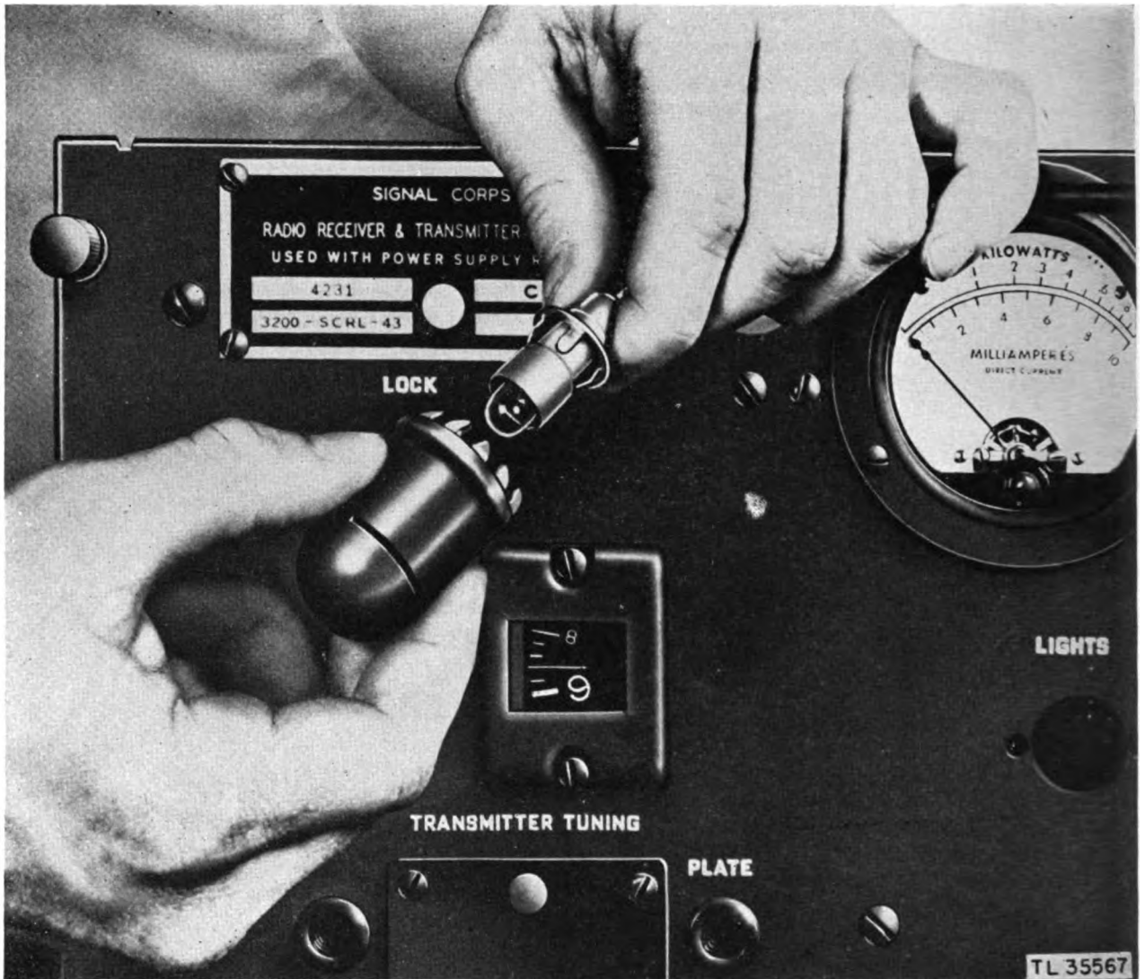
Figure 108. Radio Receiver and Transmitter BC-1267-A, meter pilot lamp removed from housing.
