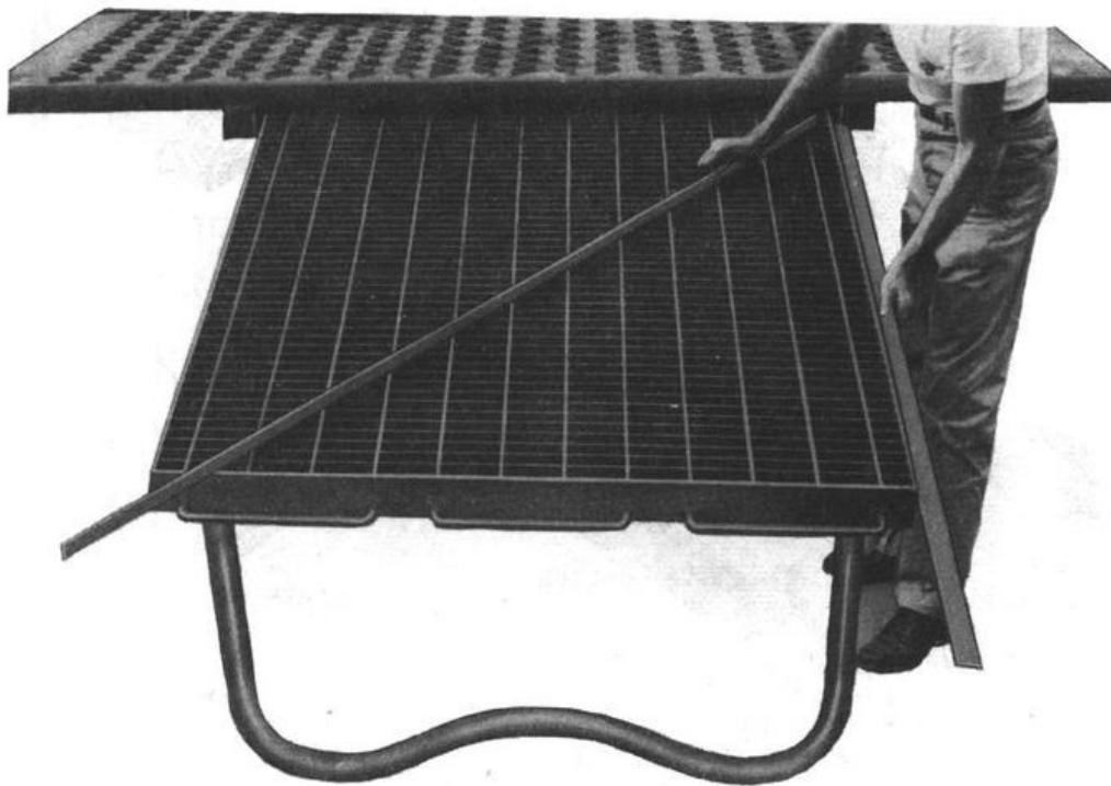
Figure 18. Checking loading ramp with straight edges
