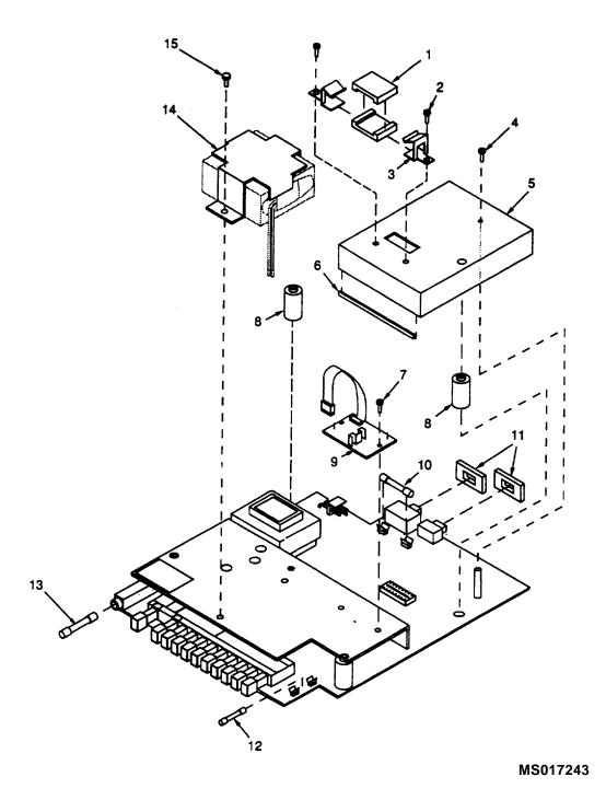
Figure 3. Motherboard Assembly A1A1
