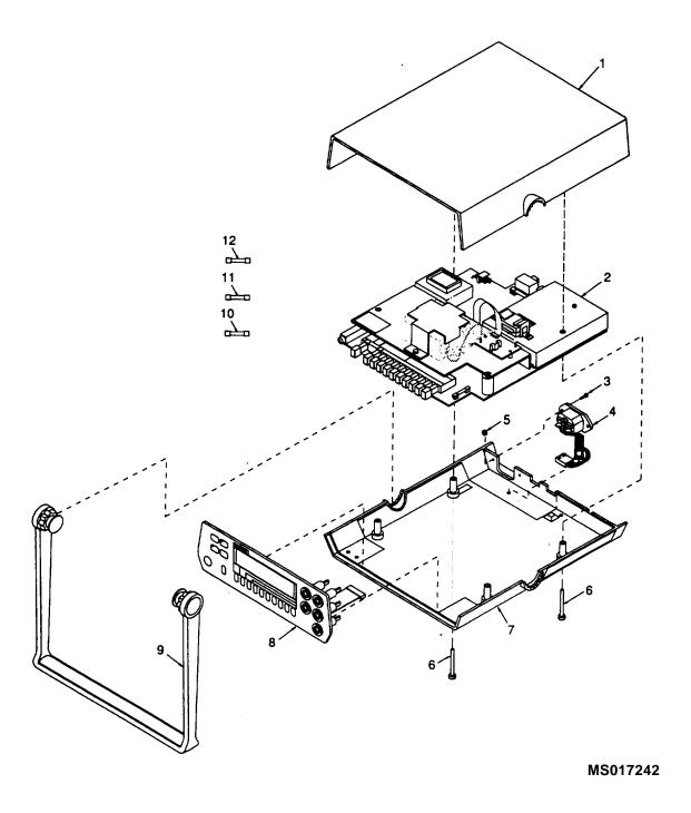
Figure 2. Digital Multimeter Assembly A1
