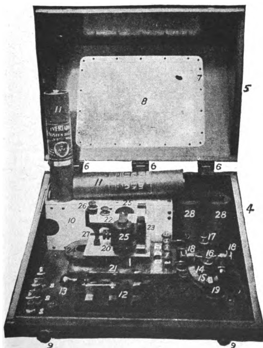
Fig. 1.—Induction telegraph set. Key to reference numbers: 1, 2, 3, binding posts; 4, case; 5, cover; 6, hinge; 7, circuit diagram frame; 8, circuit diagram; 9, cover fastener; 10, battery case; 11, tungsten, type A, battery; 12, D.P.D.T. switch; 13, switch handle; 14, key; 15, spring for key; 16, spring adjusting screw for key; 17, rear adjusting screw for key; 18, key trunnion screw and lock nut; 19, key handle; 20, sounder; 21, sounder base; 22, sounder armature; 23, sounder armature supports; 24, sounder permanent magnet; 25, coils for sounder; 26, armature movement adjusting screw; 27, spring tension adjusting screw; 28, induction coil.
