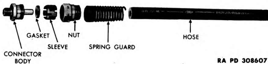
Figure 88 – Hose Assembly Disassembled
