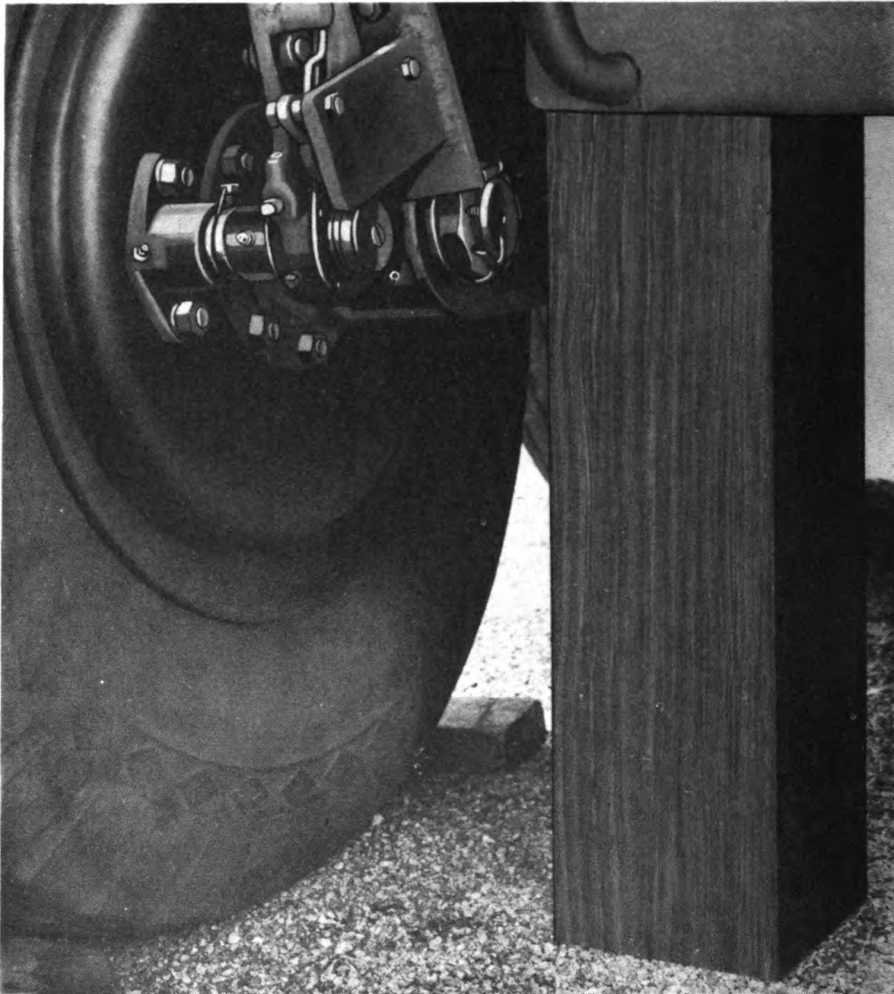
Figure 112 — Rear Corner of Body Supported for Spring Removal
