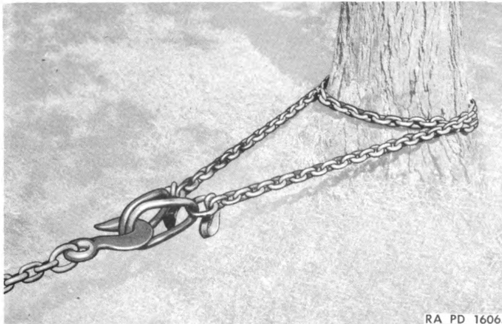
Figure 29—Correct Hitch Around Tree with Chain as used in Figures 22, 25 and 26
