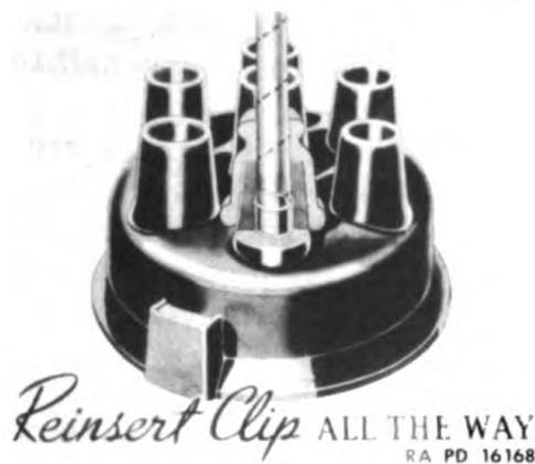
Figure 115—Installing Spark Plug Cables—Distributor Cap
