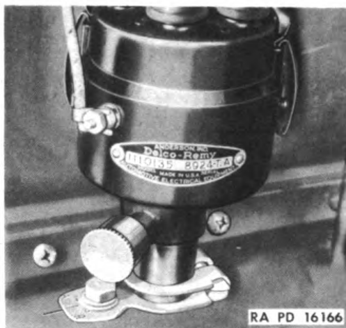
Figure 114—Distributor Manual Advance Adjustment
