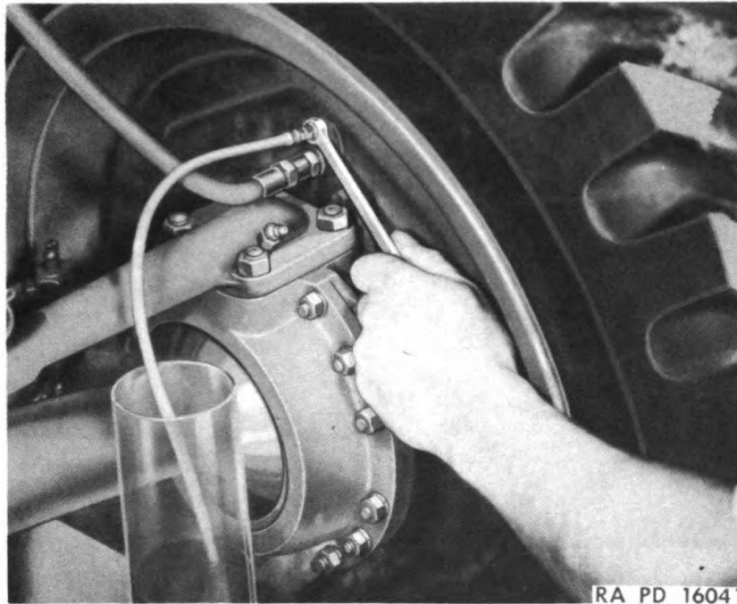
Figure 58—Typical Method of Bleeding Wheel Cylinders
