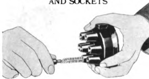
Figure 111—Cleaning Distributor Cap Socket
