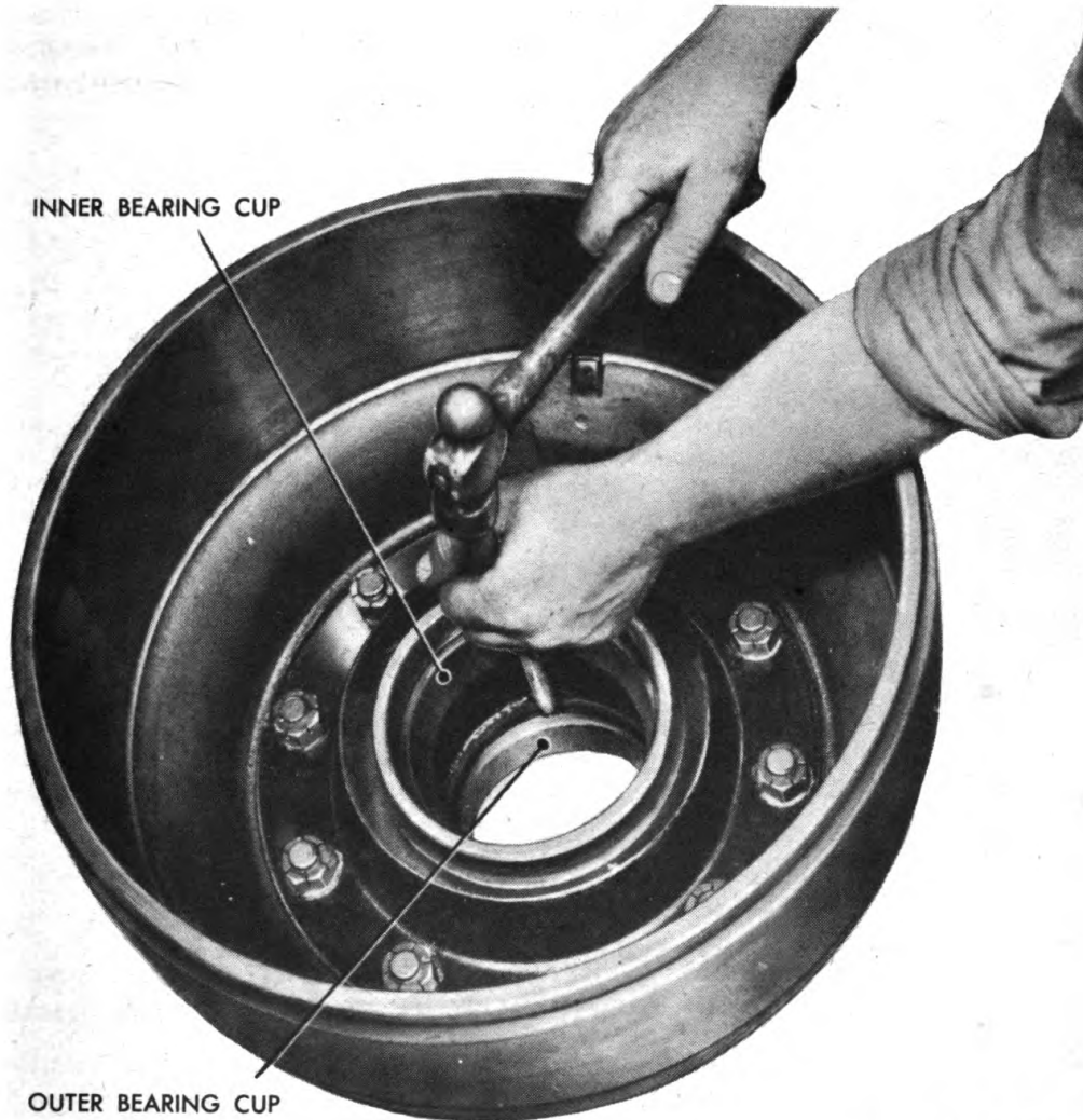
Figure 57—Removing Bearing Cups
