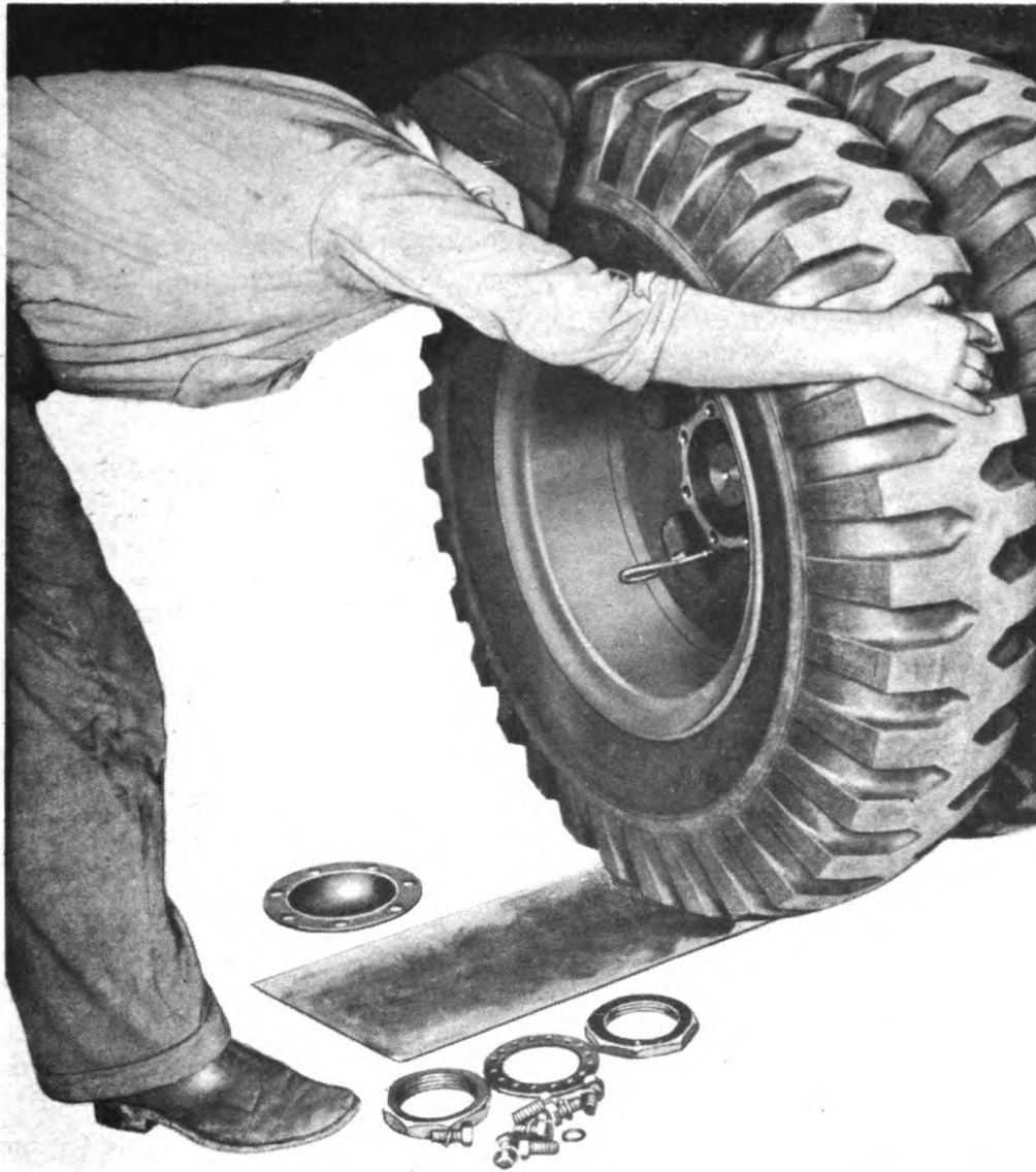
Figure 35—Removing Wheel and Hub Assembly
