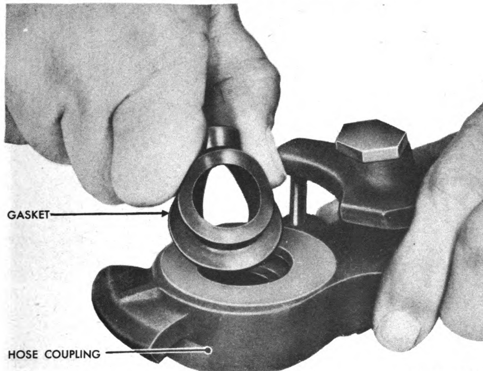
Figure 23—Installing Hose Coupling Gasket
