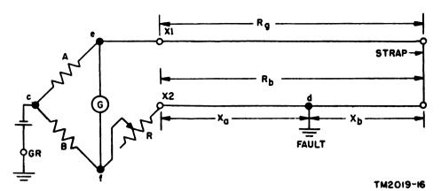
Figure 16. Regular Varley loop test circuit, simplified schematic diagram.
