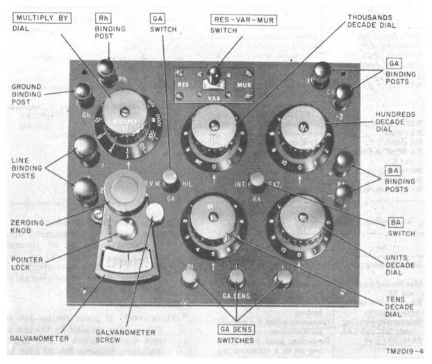
Figure 3. Operating controls, I-49, I-49-B, and ZM-4A/U.
