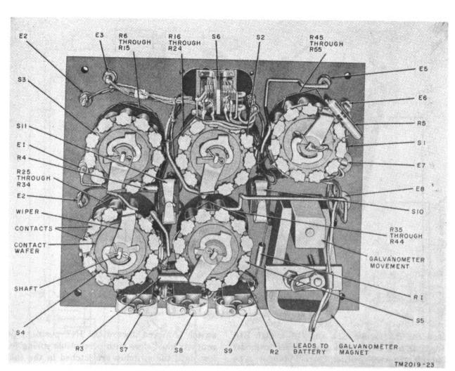
Figure 22. Resistance Bridge ZM-4A/U, bottom view.
