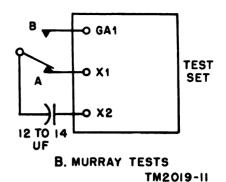
Figure 17. Connections for use of capacitor and switch to compensate for foreign voltage during test.
