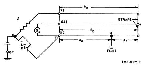
Figure 19. Hilborn loop test circuit, schematic diagram.
