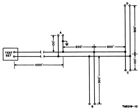
Figure 10. Branch circuit with grounded wire.
