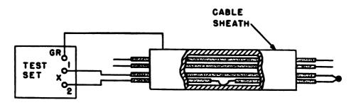
A. CONNECTIONS FOR GROUND LOCATION (SIMPLIFIED VARLEY, REGULAR VARLEY AND MURRAY LOOP TESTS)
