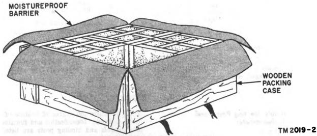
Figure 2. Typical packaging arrangement.
