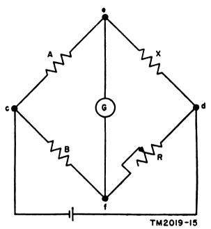
Figure 15. Basic bridge circuit.
