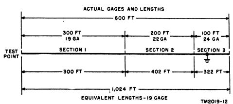
Figure 12. Grounded conductor in nonuniform gauge circuit.
