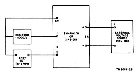
Figure 26. Test arrangement for Murray circuit test.
