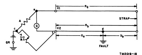
Figure 18. Murray loop test circuit, simplified schematic diagram.
