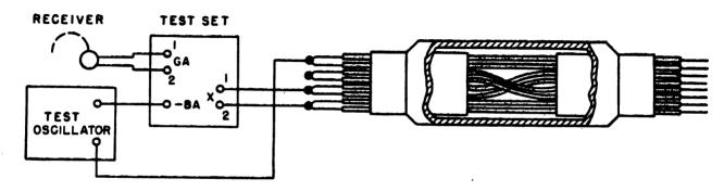
B. CONNECTIONS FOR FAULT LOCATION OF SPLIT QUADS
