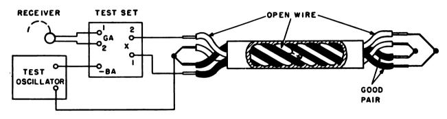
B. CONNECTIONS FOR LOCATION OF OPEN IN SPIRAL-FOUR CABLE
