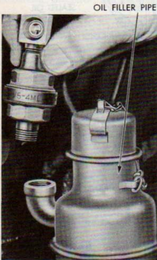
C. Installing Metering Valve
