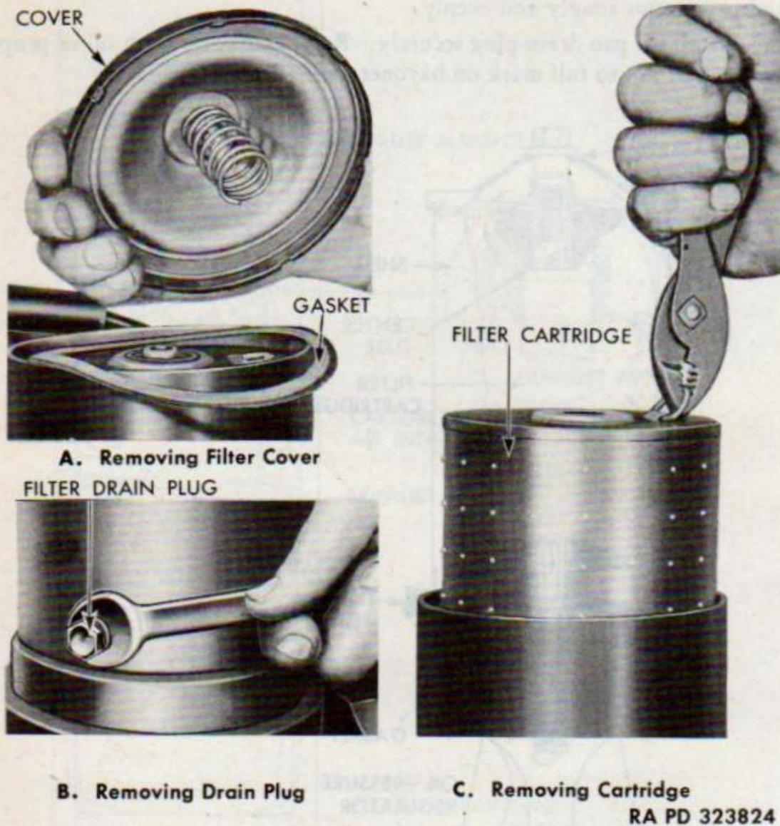
Figure 37 — Removing Oil Filter Cartridge
